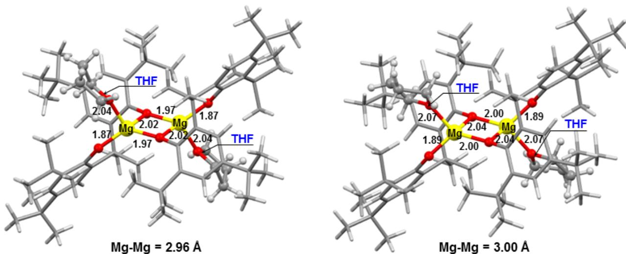
**Figure S3.** X-ray structure of [Mg(PBTP)•THF]<sub>2</sub> (left) and optimized structure from the DFT calculation (right). Bond lengths are given in Å.
