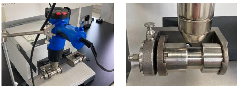
Figure S5. The set-up procedure for a heat gun on MM400.
