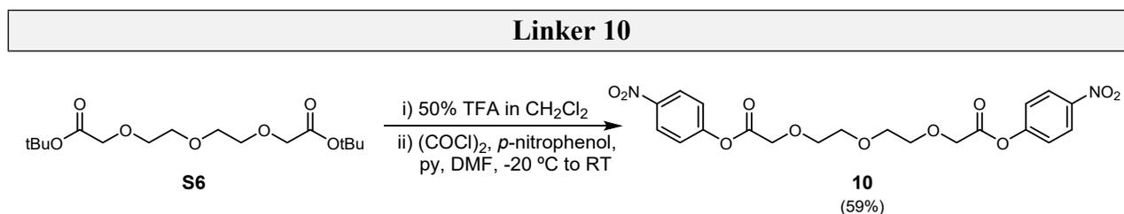
**Scheme S3** Synthesis of *p*-nitrophenyl activated linker **10**.
