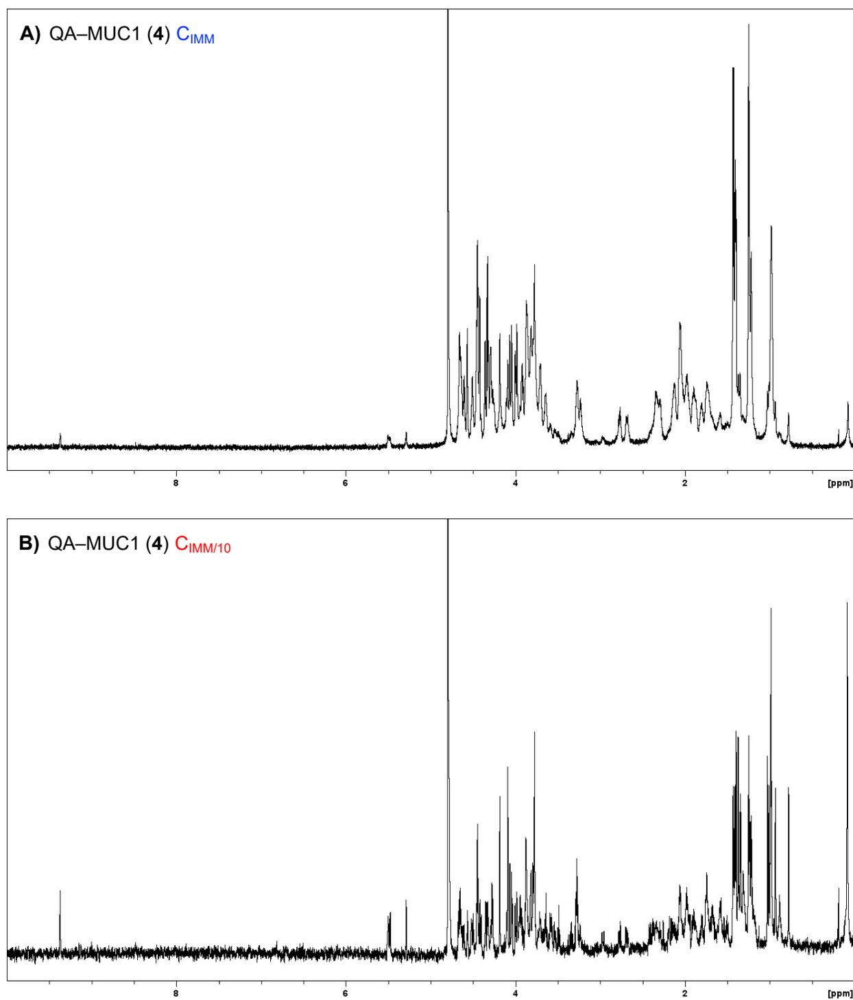
**Fig. S55**  $^1\text{H}$ -NMR spectra (800 MHz) of QA-MUC1 **4** (PBS/ $\text{D}_2\text{O}$ ) at (A) the immunization concentration ( $C_{\text{IMM}} = 0.337$  mM) and (B) ten-fold diluted sample ( $C_{\text{IMM}/10} = 0.0337$  mM).
