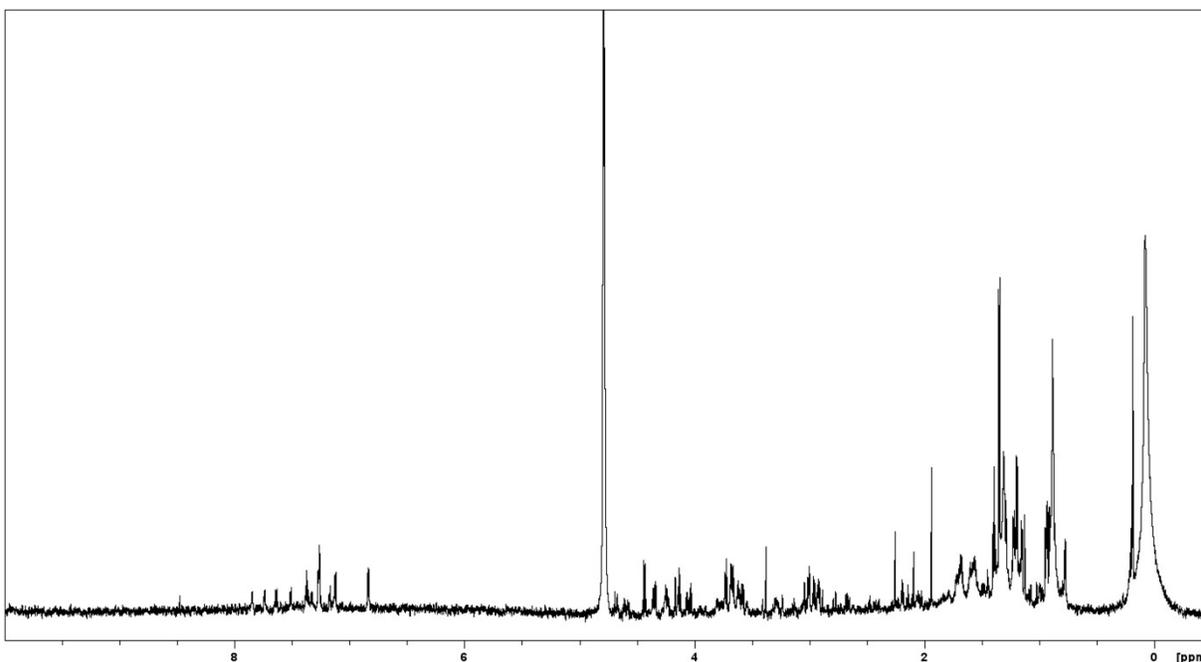
**Fig. S38** <sup>1</sup>H-NMR spectrum of PV peptide **S8** (30 μM, PBS/D<sub>2</sub>O, 298 K, 800 MHz).
