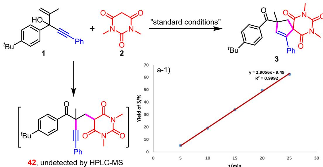
In a 15 mL oven-dried pressure sealed tube, a mixture of 1,4-enyne **1** (304.2 mg, 1 mmol), 1,3-dimethylbarbituric acid **2** (234.1 mg, 1.5 mmol), Ag<sub>2</sub>O (459.6 mg, 2 mmol), and acetonitrile (3 mL) was heated to 110 °C. Aliquots of 0.1 mL were removed from the cell every 5 minutes and the yields of the product were determined by HPLC analysis with **3** as the external standard.
