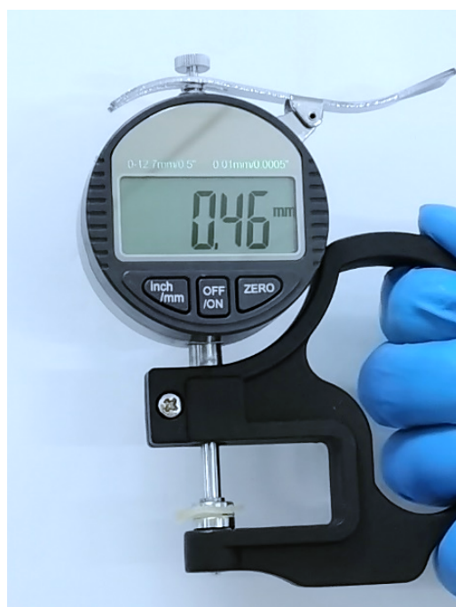
Figure S12. Thickness of IC-Zn gel electrolyte used to measure ionic conductivity.
