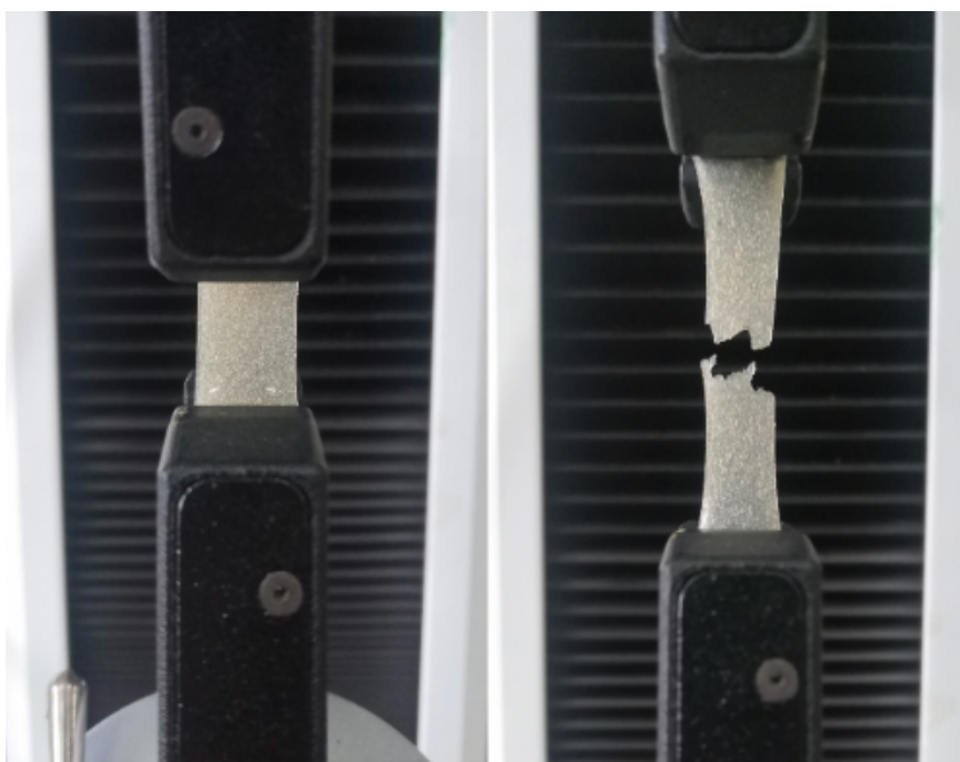
Figure S4. Optical photographs of IC-Zn-36 gel electrolyte before and after tensile test.
