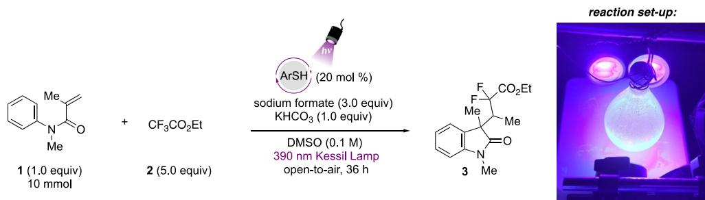
**Figure S3.** Reaction conditions and set-up.
