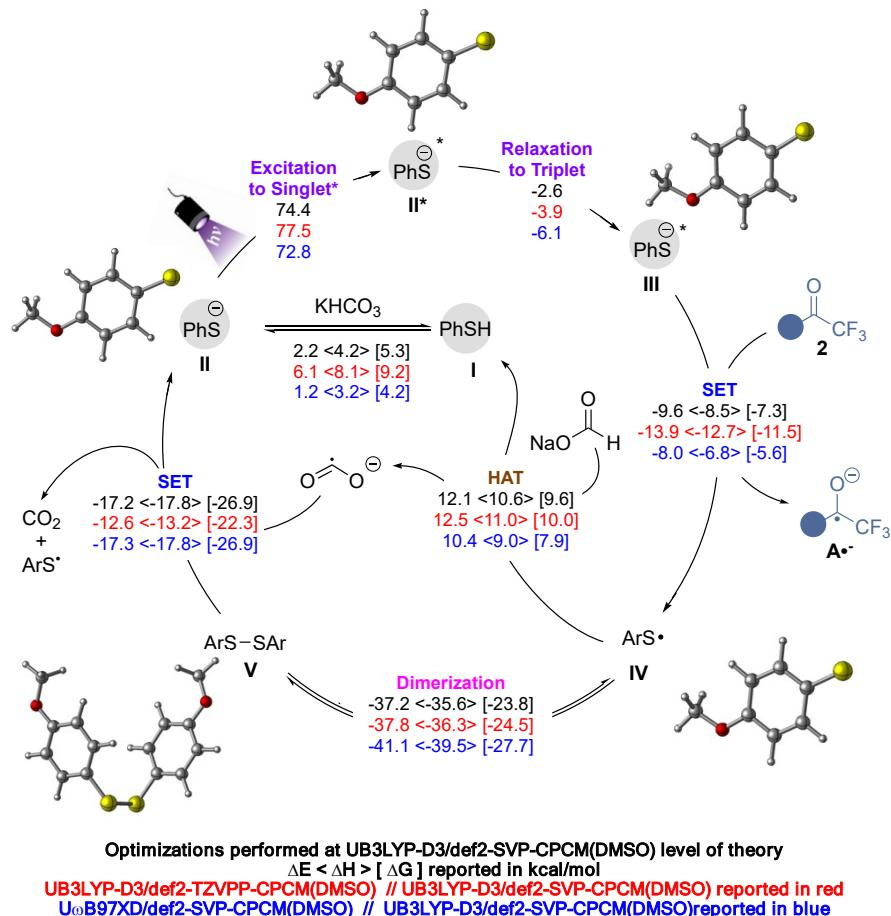
**Figure S8.** Energetics of thiolate catalytic cycle. Optimizations performed at UB3LYP-D3/def2-SVP-CPCM(DMSO) level of theory,  $\Delta E < \Delta H$  in angle brackets > [ $\Delta G$  in square brackets] for each relevant step reported in kcal/mol. Single point energies are also shown.
