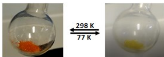
Fig. S5.1| Thermochromism exhibited by single crystals of DMP crystals at 77 K and 298 K, respectively.
