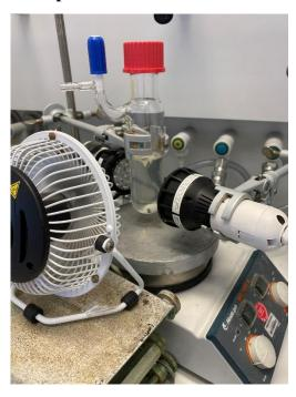
**Fig. S9.** Reaction setup used for the large scale synthesis of **57** featuring two 18 W blue LEDs ( $\lambda_{\text{max}} = 405 \text{ nm}$ ).
