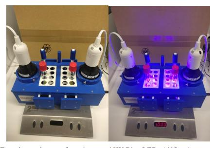
**Fig. S8.** Experimental set-up featuring two 18W Blue LEDs (405 nm).
