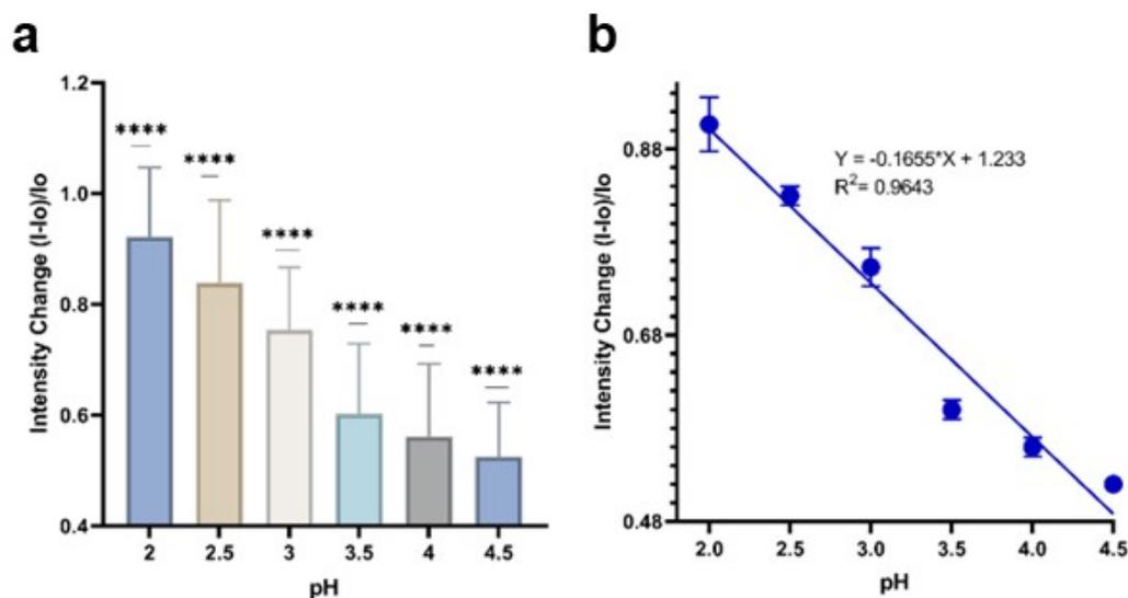
**Figure S7.** Optical responses from PDADMAC-SDBS-SWCNTs in artificial sweat at various pH ranges (pH 2 - 4.5),  $n = 3$  a) Intensity changes and b) pH response curve showing line with
