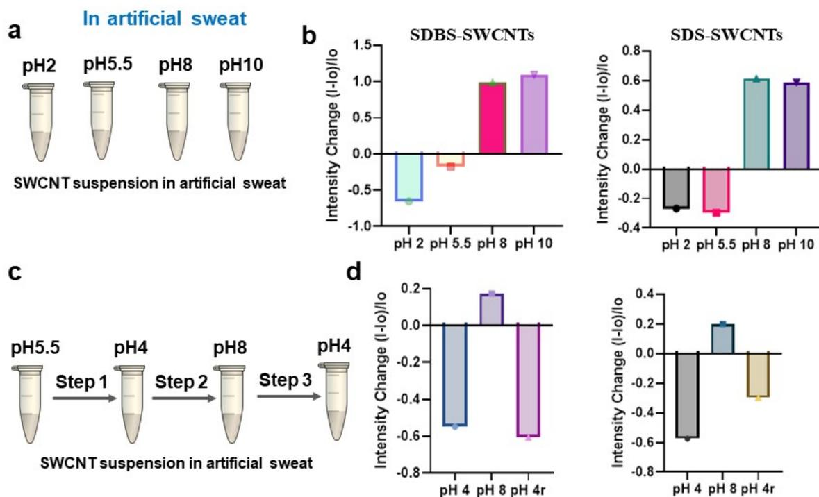
**Figure S6.** Optical responses in artificial sweat from SDS-SWCNTs at various pH ranges (pH 2-10) a) Schematic illustration of the process, b) Intensity changes at various pH as represented in a, c) Schematic for sequential in situ pH changes, d) Intensity changes in sequential in situ pH changes as represented in c, pH 4r represents solution pH reversed to pH4 from pH 8,  $n=3$ .
