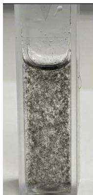
**Figure S3.** Aggregation of SC-SWCNTs at pH 4.
