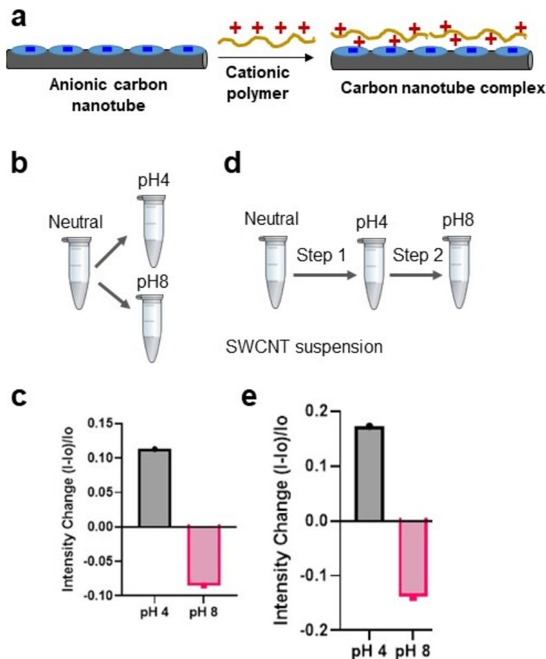
**Figure S5.** Surface chemistry modulation on nanotubes and optical responses from PDADMAC-SDS-SWCNT at various pH a) Schematic illustration of surface chemistry modulation by adding a cationic polymer, b) Schematic illustration of direct pH changes, c) Intensity changes of PDADMAC-SDS-SWCNTs from direct pH changes represented in b, d) Schematic illustration of in situ pH changes, e) Intensity changes of PDADMAC-SDS-SWCNTs from in situ pH changes represented in d,  $n=3$ .
