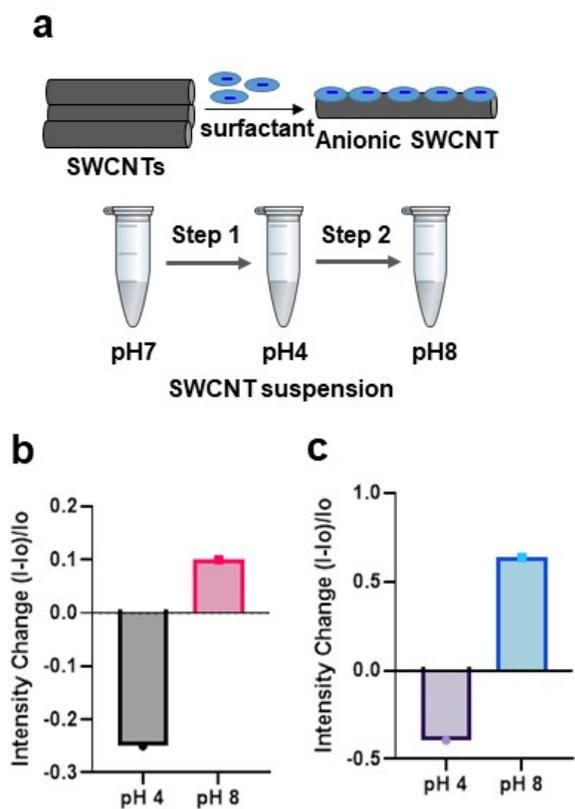
**Figure S4.** Optical responses from nanotubes for in situ pH ranges a) Schematic illustration of the process, b) Intensity changes of SDS-SWCNTs, c) Intensity changes of SDBS-SWCNTs,  $n=3$ .
