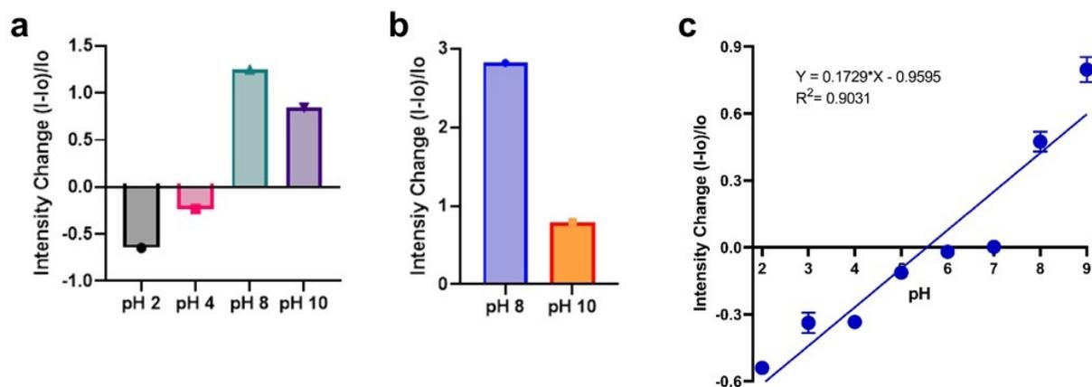
**Figure S2.** Fluorescence intensity of SWCNT suspension a) SDS-SWCNTs and b) SC-SWCNTs. c) pH-response curve via intensity changes of SDBS-SWCNTs. Solid line represents linear regression fits,  $n=3$ .
