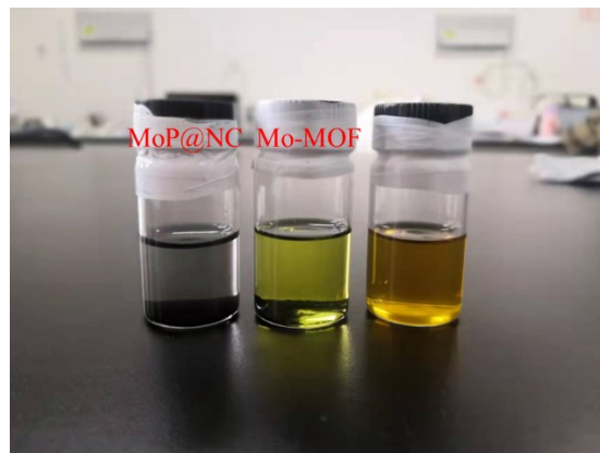
Fig. S12 Photograph of blank, MoP@NC and Mo-MOF immersed in \text{Li}_2\text{S}_6 solution after 2 h.
