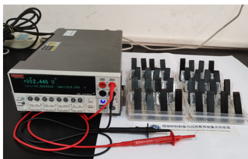
Fig. S13. The photograph of the 32 WHEGs system in series connections.
