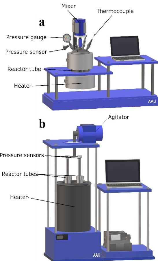
**Figure S1.** Schematic view of a) HTL and b) HT setups.
