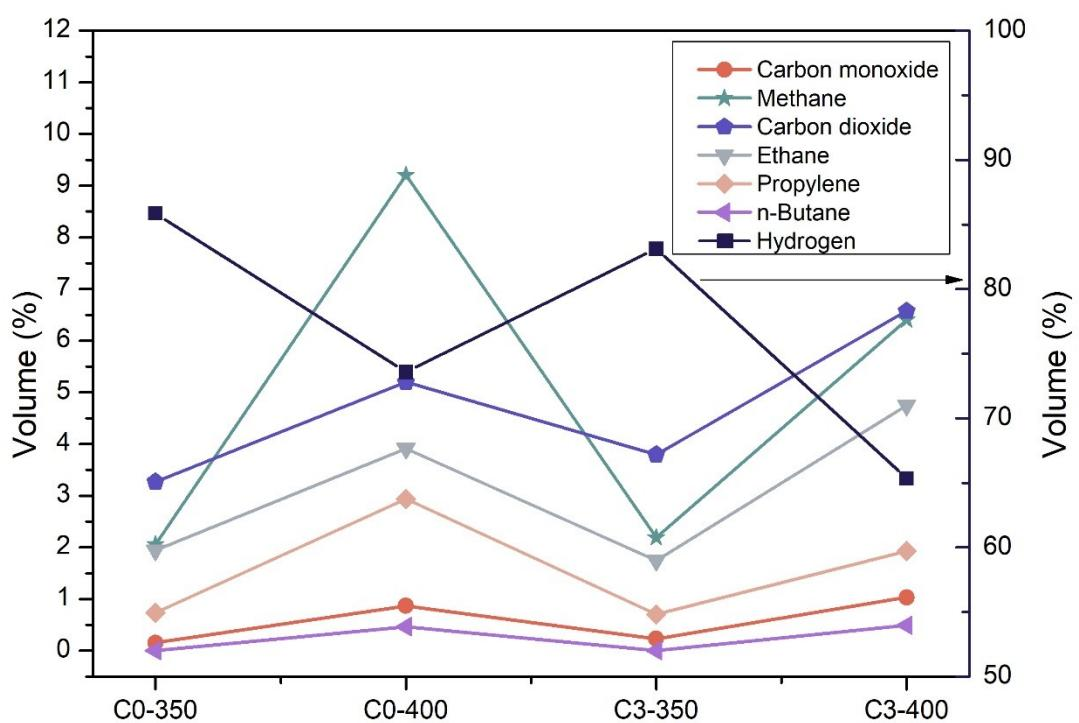
**Figure S3.** The gas composition of HT experiments.
