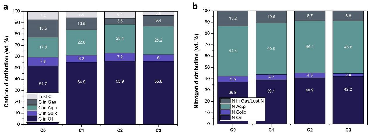
**Figure S4.** a) Carbon and b) Nitrogen distribution among different HTL products.
