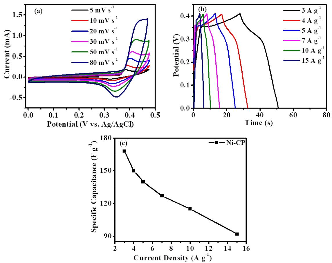
**Fig. S13** (a) CV curves at various scan rate from 5 to 80  $\text{mV s}^{-1}$  (b) GCD curves at different current density from 3 to 15  $\text{A g}^{-1}$  (c) Specific capacitance of Ni-CP (1M LiOH).
