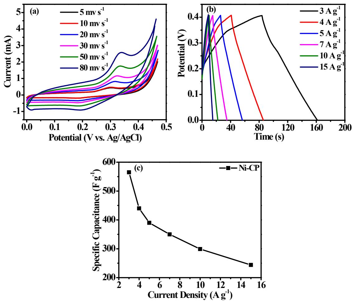
**Fig. S9** (a) CV curves at various scan rate from 5 to 80  $\text{mV s}^{-1}$  (b) GCD curves at different current density from 3 to 15  $\text{A g}^{-1}$  (c) Specific capacitance of Ni-CP (5M KOH).
