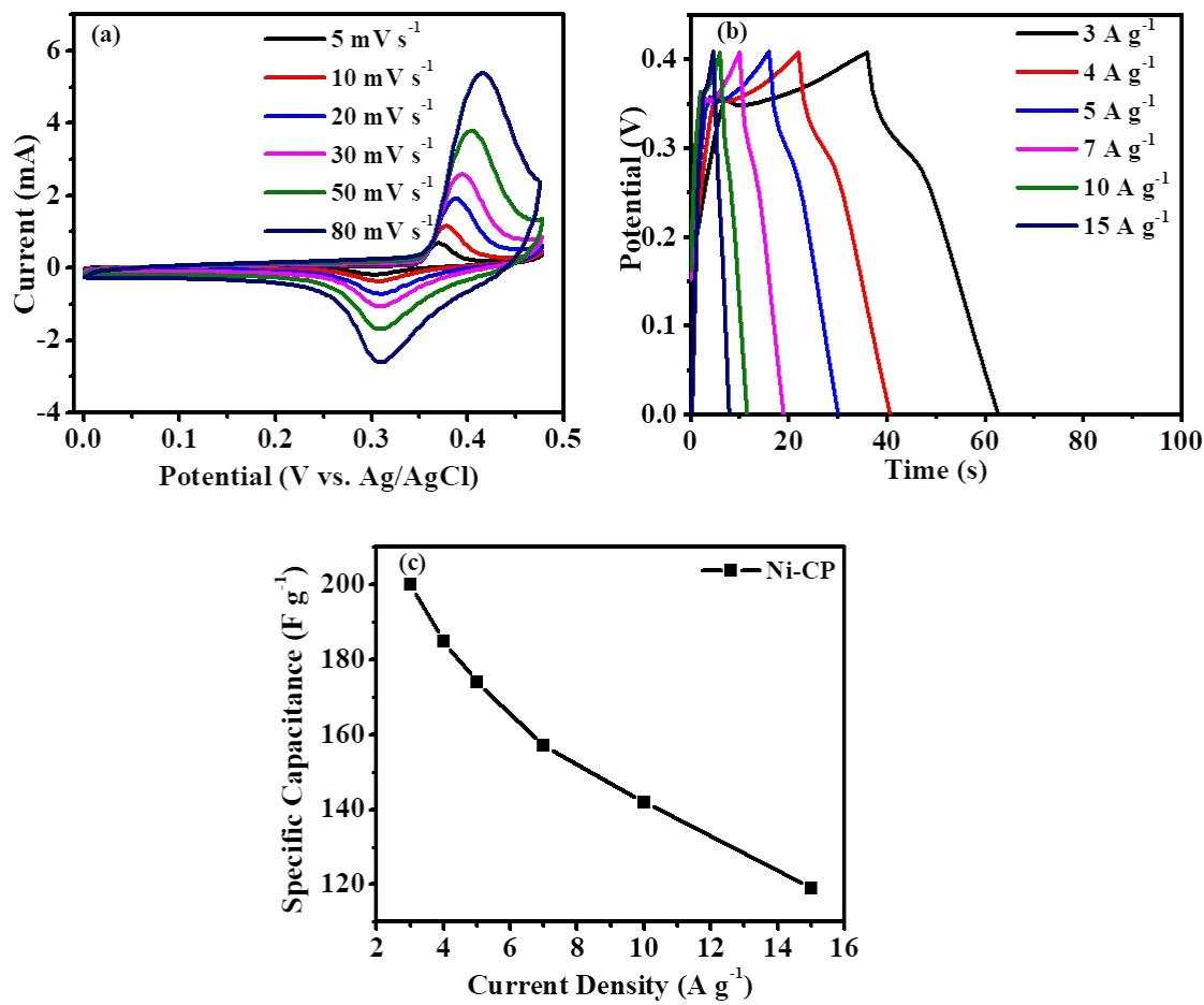
**Fig. S11** (a) CV curves at various scan rate from 5 to 80 mV s<sup>-1</sup> (b) GCD curves at different current density from 3 to 15 A g<sup>-1</sup> (c) Specific capacitance of **Ni-CP** (1M KOH).
