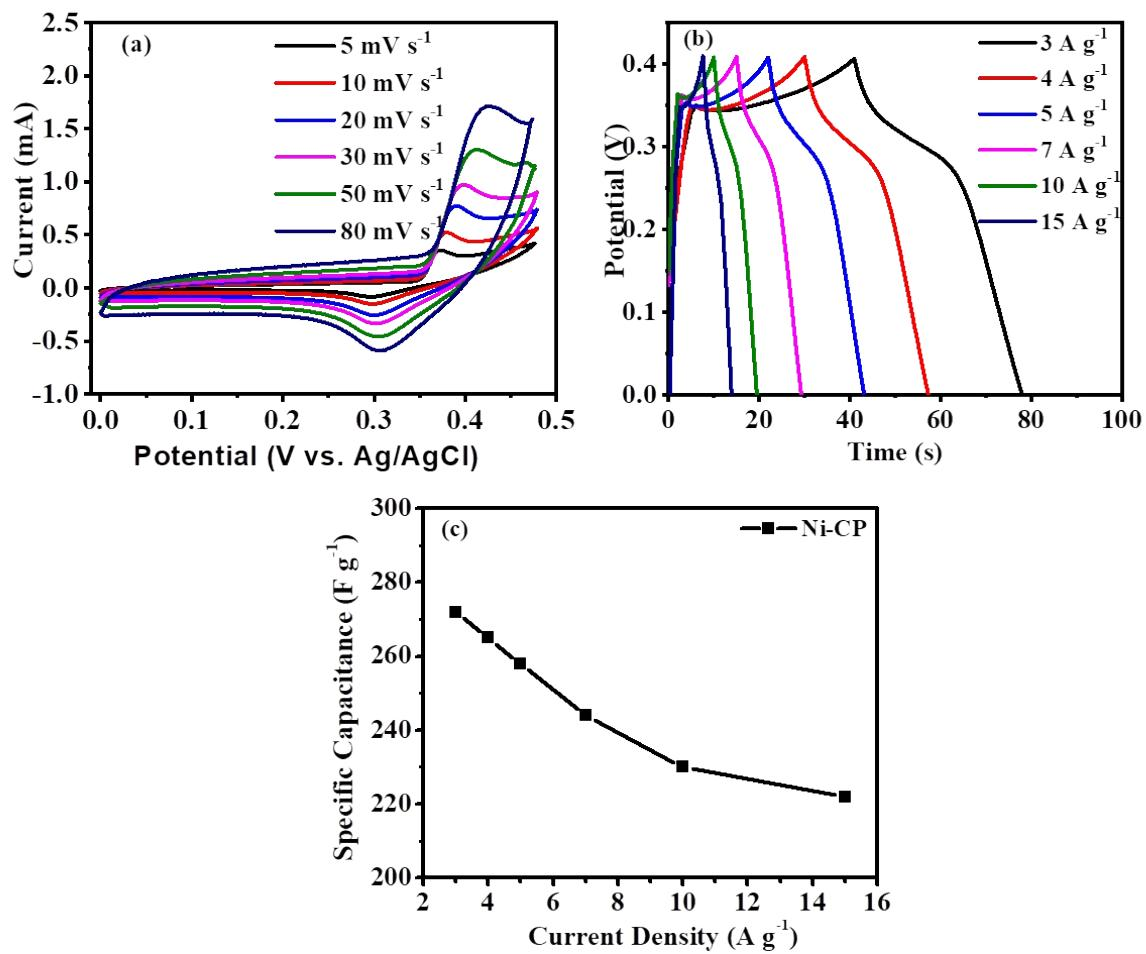
**Fig. S12** (a) CV curves at various scan rate from 5 to 80 mV s<sup>-1</sup> (b) GCD curves at different current density from 3 to 15 A g<sup>-1</sup> (c) Specific capacitance of Ni-CP (1M NaOH).
