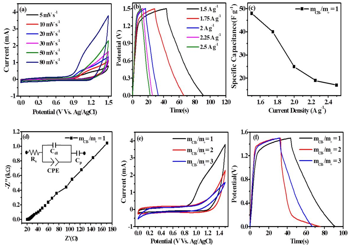
**Fig. S14** (a) CV curves at various scan rate from 5 to 80 mV s<sup>-1</sup> (b) GCD curves at different current density from 1.5 to 2.5 A g<sup>-1</sup> (c) Specific capacitance, (d) EIS of ASC device of Ni-CP of  $m_{CB}/m_+ = 1$ , (e) and (d) Comparison of CV (at 80 mV s<sup>-1</sup>) and GCD (at 1.5 A g<sup>-1</sup>) curve of different mass loading of positive and negative electrode materials ( $m_{CB}/m_+ = 1$ ,  $m_{CB}/m_+ = 2$ ,  $m_{CB}/m_+ = 3$ )
