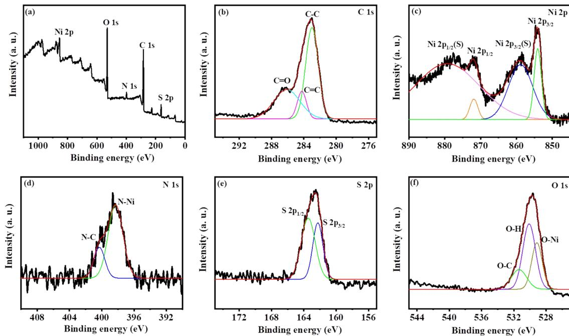
**Fig. S7** (a) XPS survey spectrum (b-f) corresponding high resolution spectra of C 1S, Ni 2P, N 1S, S 2P and O 1S of **Ni-CP**.
