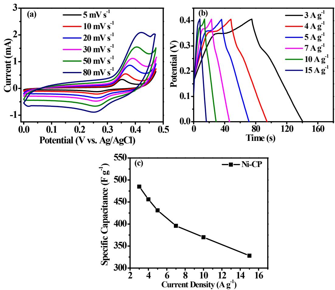
**Fig. S10** (a) CV curves at various scan rate from  $5$  to  $80 \text{ mV s}^{-1}$  (b) GCD curves at different current density from  $3$  to  $15 \text{ A g}^{-1}$  (c) Specific capacitance of Ni-CP (3M KOH).
