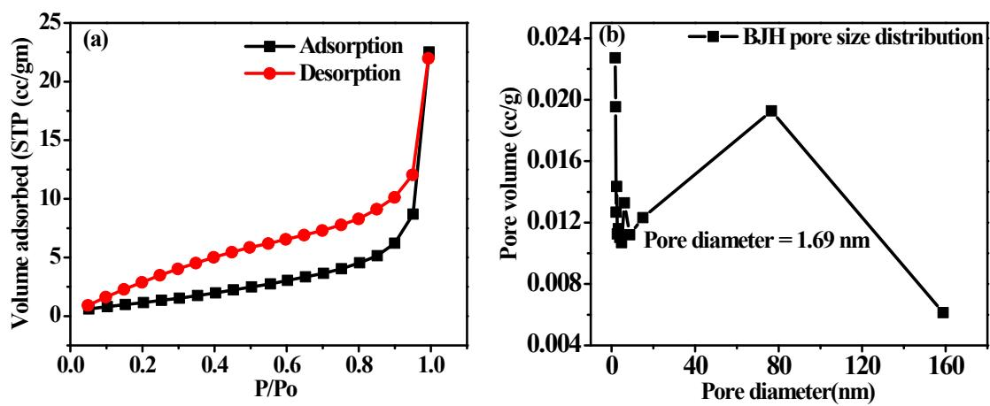
**Fig. S8** (a) Nitrogen adsorption and desorption isotherms and (b) the corresponding microporous analysis of **Ni-CP**.
