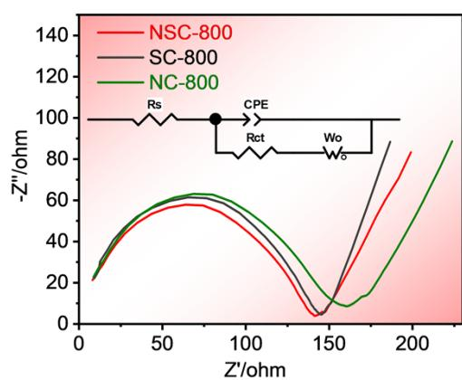
**Fig. S8** Nyquist plots of NSC-800, SC-800 and NC-800, with the inset showing the equivalent circuit for fitting the experimental data.
