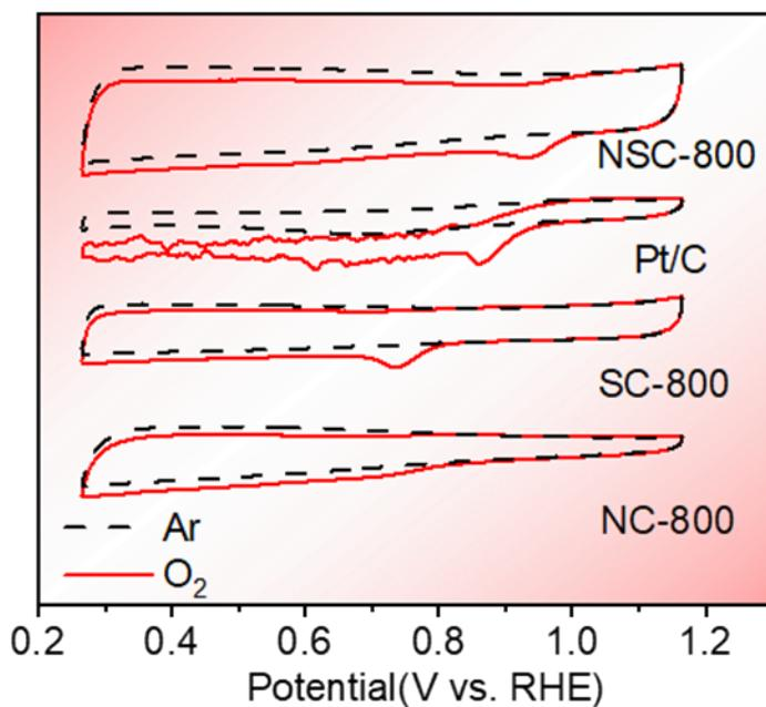
**Fig. S5** CV tests for NSC-800, SC-800, NC-800, and Pt/C under Ar and O<sub>2</sub> saturated 0.1 m KOH.
