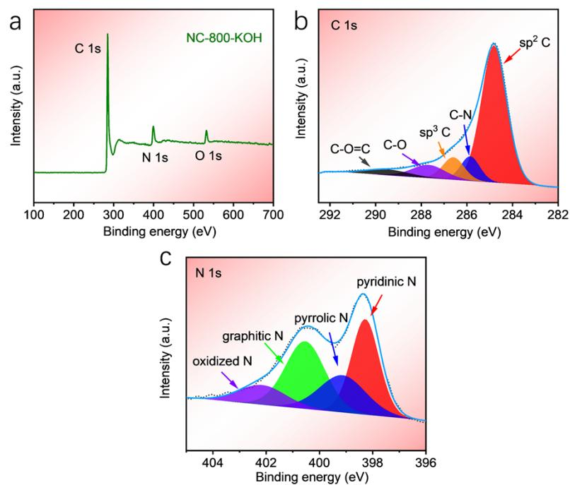
**Fig. S11** (a) XPS survey spectra. High-resolution XPS spectra of (b) C 1s and (c) N 1s peaks for NC-800-KOH.
