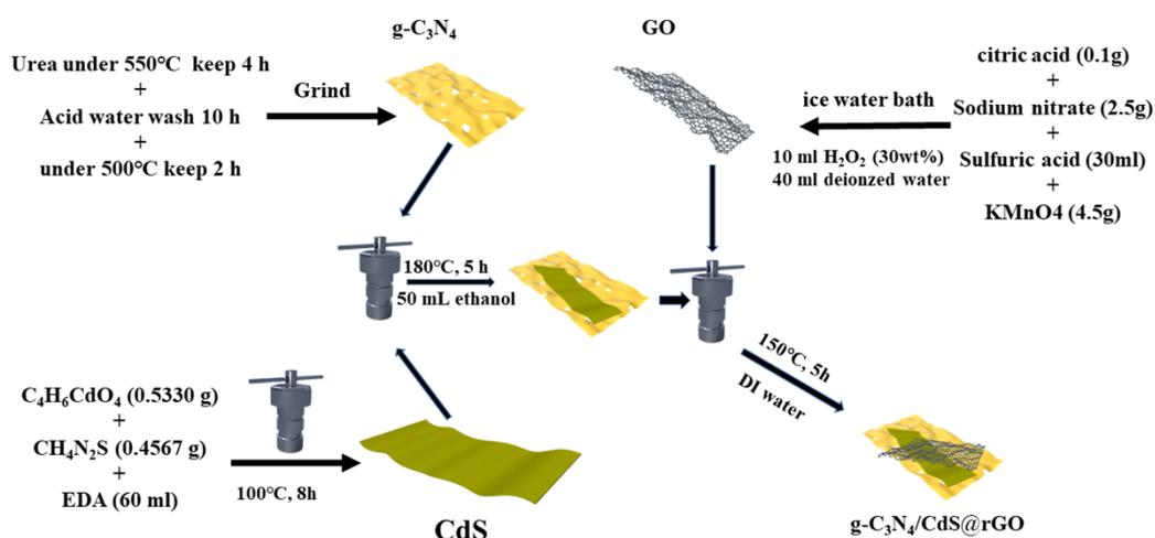
**Scheme. 1** The schematic diagram of the synthetic route of CN/CdS@rGO.
