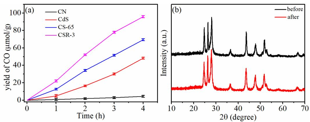
**Figure. S6** (a) Deviation analysis of CO yield. (b) The XRD of CSR-3 before and after  $\text{CO}_2$  reduction experiment.
