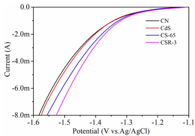
**Figure. S4** The LSV spectra of CN, CdS, CS-65 and CSR-3.
