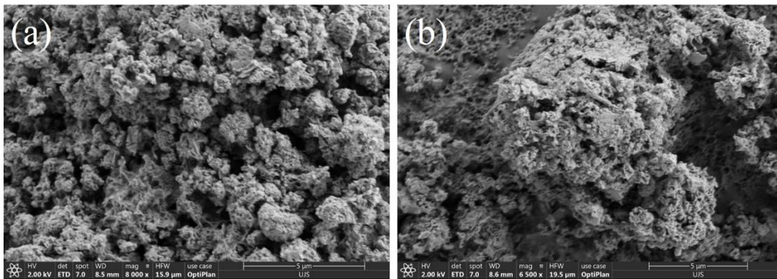
**Figure. S8** The SEM of (a) CdS, (b) CSR-3 of after cycling experiment.
