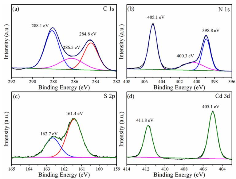
**Figure. S7** XPS of CSR-3 after cycling experiment.
