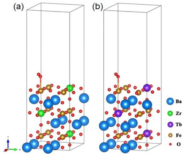
Figure 3.  $O_2$  adsorption model for (a) BZF and (b) BTF.
