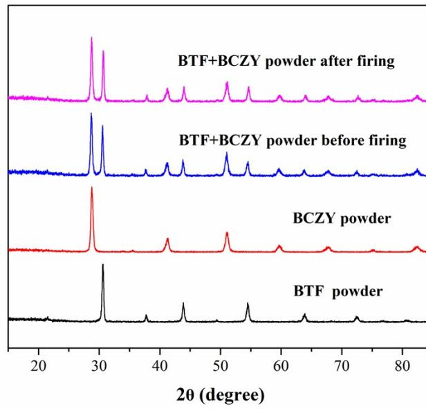
Figure 4. XRD patterns for BTF+BCZY composite powder before and after firing. The XRD patterns for BTF and BCZY are also added as the reference.
