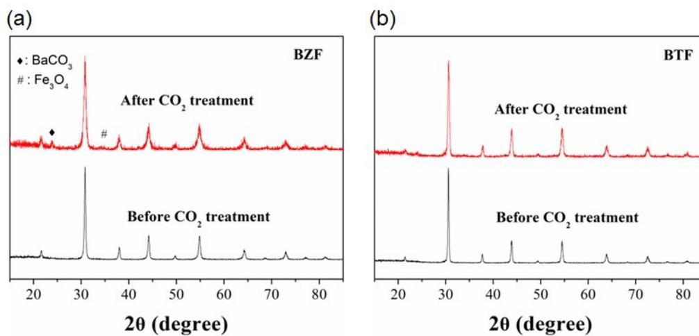
Figure S1. XRD patterns for (a) BZF and (b) BTF before and after the treatment in 20% CO<sub>2</sub> at 600 °C for 10 h.
