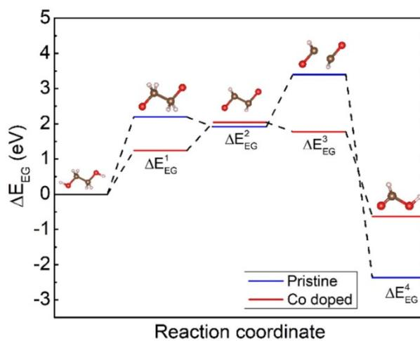
**Figure S11.** The calculated energy landscape of the EG electrooxidation reaction process on the pristine and Co doped  $\text{Ni}_2\text{P}$  surfaces.
