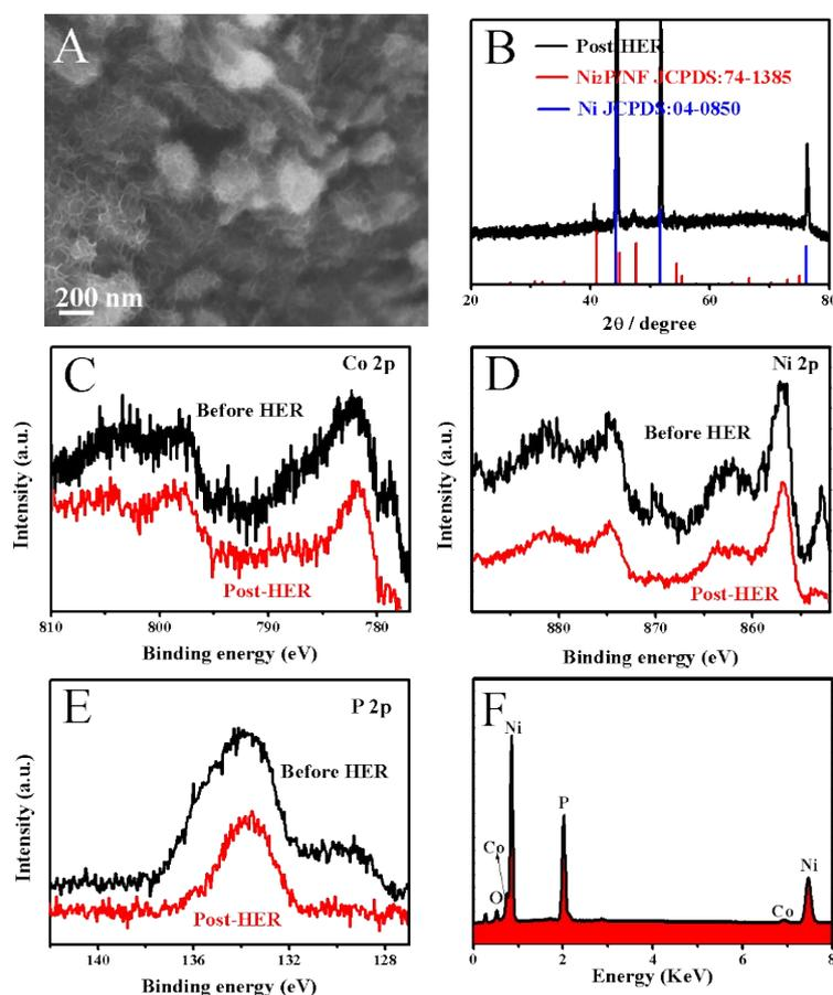
**Figure S6.** The morphology characterization and composition analyses of Co<sub>0.6</sub>-Ni<sub>2</sub>P/NF after HER reaction. (A) the SEM image, (B) XRD pattern, high-resolution XPS spectra of (C) Co 2p, (D) Ni 2p, (E) P 2p peaks of the Co-Ni<sub>2</sub>P/NF and (F) SEM-EDS spectral of the Co-Ni<sub>2</sub>P/NF.
