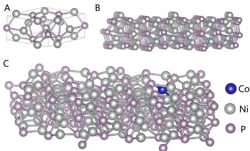
**Figure S4.** The atomic models of Ni<sub>2</sub>P unitcell. (A) pristine surface (B) and Co doped surface.
