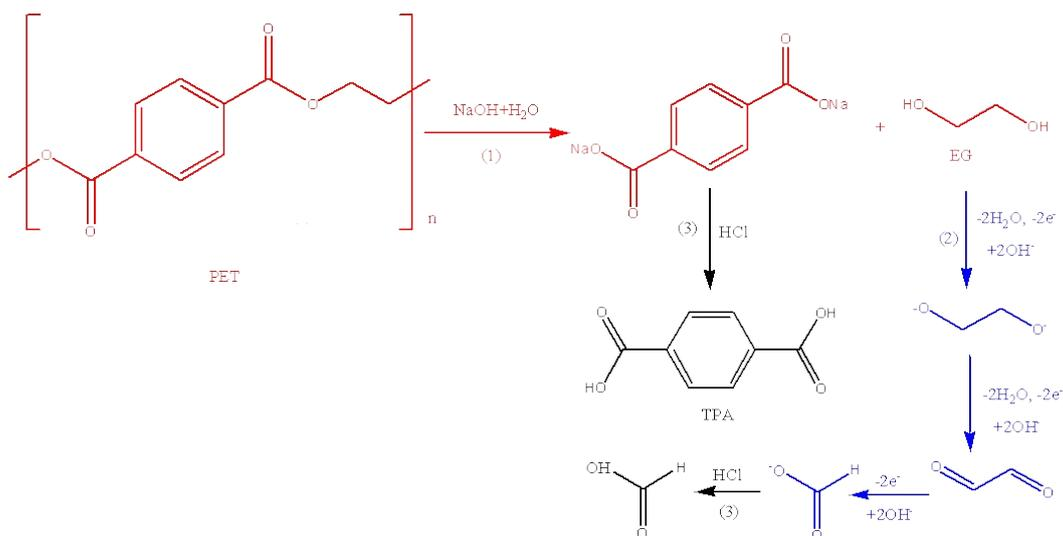
**Figure S9.** The process for waste PET bottle upcycling.
