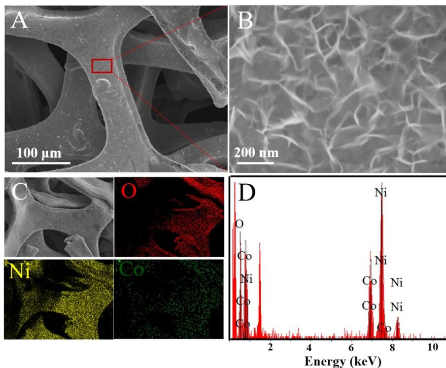
**Figure S1.** Morphological and composition characterizations of Co-Ni(OH)<sub>2</sub>/NF. (A) and (B) SEM images, (C) SEM-mapping, and (D) SEM-EDX.
