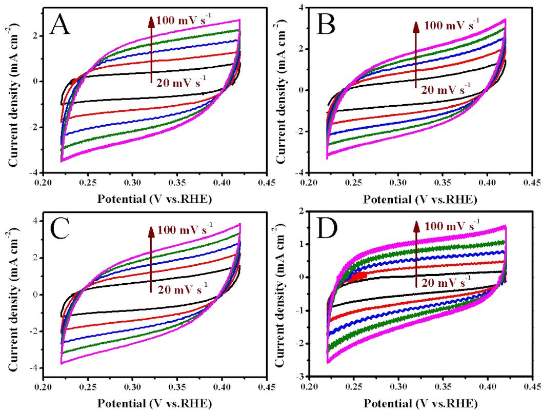
**Figure S3.** CV curves of (A) Co<sub>0.6</sub>-Ni<sub>2</sub>P/NF, (B) Ni<sub>2</sub>P/NF, (C) CoP/NF, and (D) Co-Ni(OH)<sub>2</sub>/NF in 1 M NaOH electrolyte at different scan rates.
