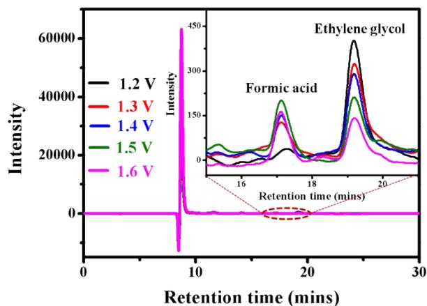
**Figure S7.** The HPLC analysis of the products of PET hydrolysate electrooxidation.
