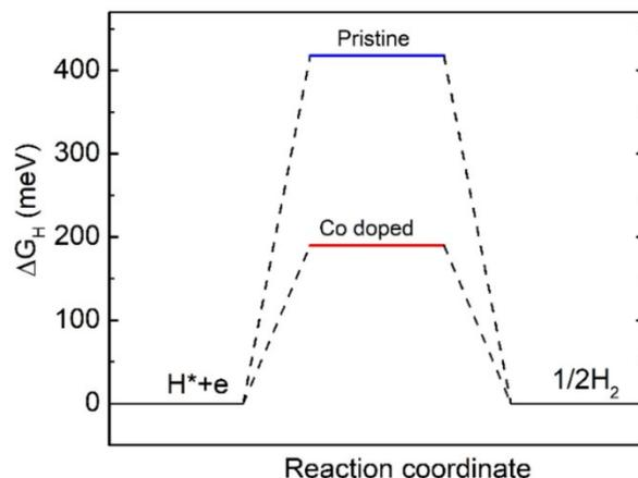
**Figure S5.** The calculated Gibbs free energies of H on the pristine and Co doped Ni<sub>2</sub>P surfaces.
