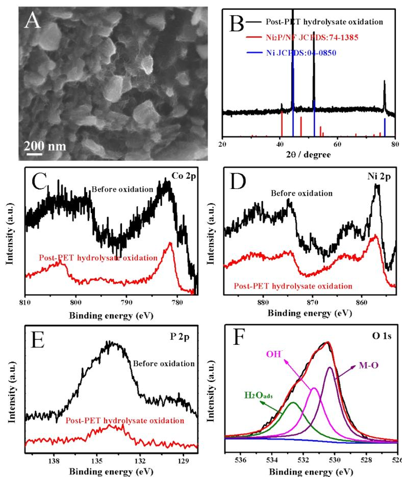
**Figure S8.** The morphology characterization and composition analyses of Co-Ni<sub>2</sub>P/NF post-PET hydrolysate electrooxidation. (A) the SEM image, (B) XRD pattern, high-resolution XPS spectra of (C) Co 2p, (D) Ni 2p, (E) P 2p and (F) O 1s peaks of the Co-Ni<sub>2</sub>P/NF.
