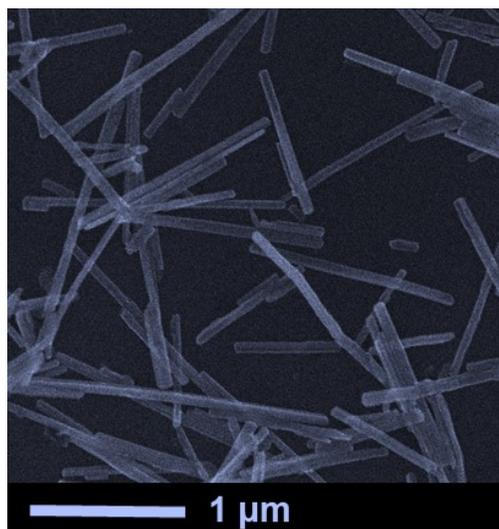
**Fig. S8** SEM images of CdS-P<sub>0.8</sub> NRs after photocatalytic hydrogen production under blue LED light irradiation using lactic acid as a sacrificial agent.
