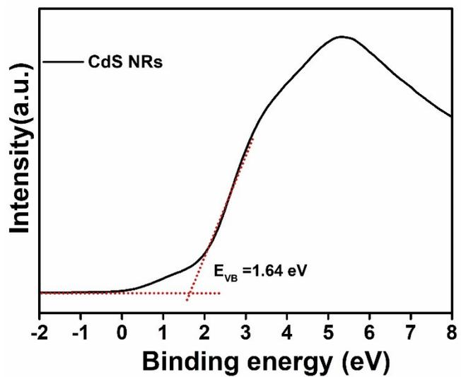
**Fig. S9** Valence band XPS spectra of CdS-P<sub>0.8</sub> NRs.
