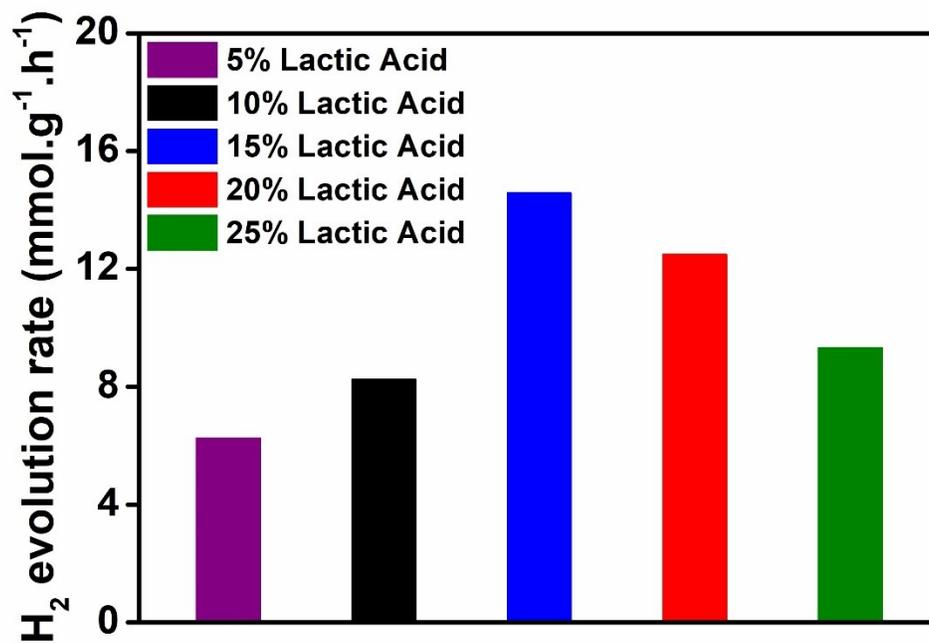
**Fig.S6** Effect of lactic acid concentration on H<sub>2</sub> evolution performance of CdS-P<sub>0.8</sub> NRs.
