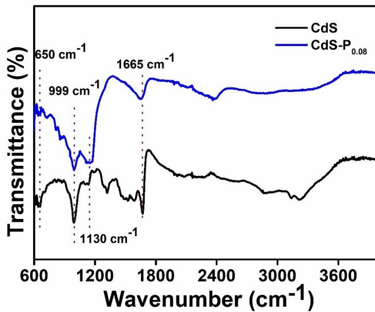
**Fig. S3** FTIR spectra of pristine CdS and CdS- $\text{P}_{0.8}$  NRs samples.
