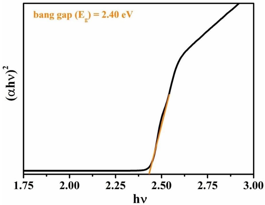
**Fig. S4** Band gap energy plot from UV–Vis diffuse reflectance spectrum of the CdS NRs.
