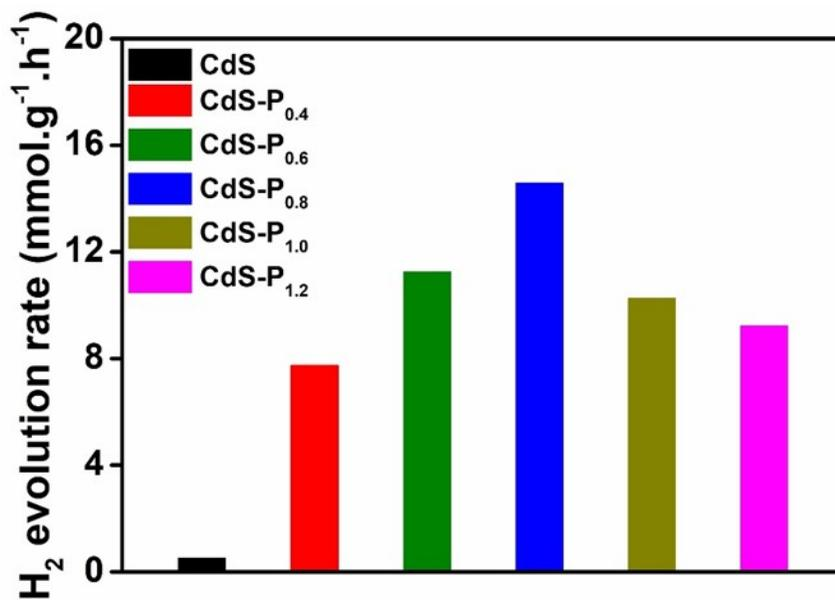
**Fig. S5** Hydrogen evolution rates of a series of CdS-P and CdS NRs under blue LED light irradiation using 15 vol% lactic acid as a sacrificial agent.
