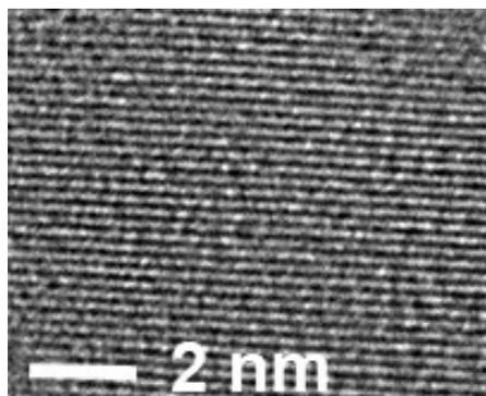
**Fig. S1** HR-TEM images of (E) CdS NRs, indicating the crystal structure of hexagonal CdS nanorods.
