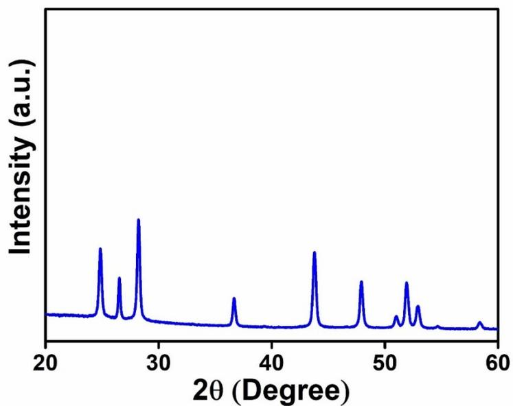
**Fig. S7** XRD patterns of CdS-P<sub>0.8</sub> NRs after photocatalytic hydrogen production under blue LED light irradiation using lactic acid as a sacrificial agent, indicating that this results were well-matched of the CdS-P<sub>0.8</sub> NRs before and after photocatalytic hydrogen production reactions.
