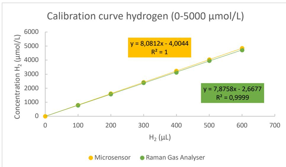
**Figure S3.** Calibration curve for 0 – 600 μL of hydrogen added to an Ar-flushed 4.9 mL glass vial.
