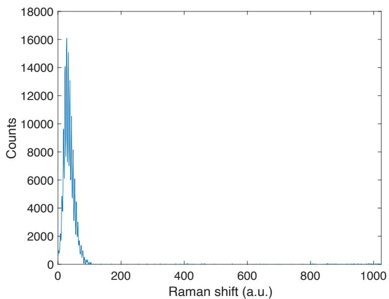
**Figure S10.** Spectral signature of CO<sub>2</sub> recorded with the Raman Gas analyser.
