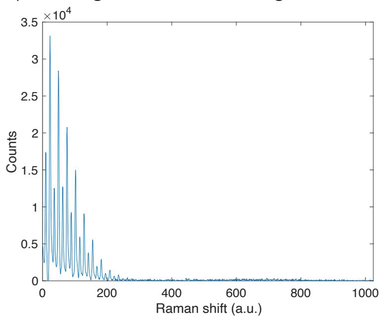
**Figure S8.** Spectral signature of N<sub>2</sub> recorded with the Raman Gas analyser.
