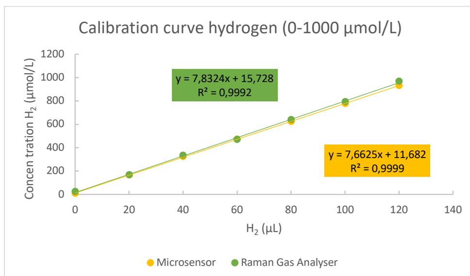
**Figure S2.** Calibration curve for 0 – 120 µL of hydrogen added to an Ar-flushed 4.9 mL glass vial.
