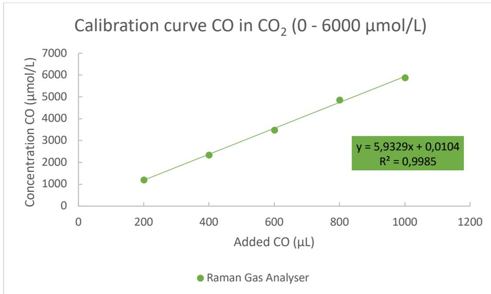
**Figure S6.** Calibration curve for 0 – 1000 µL of CO added to a CO<sub>2</sub>-flushed 4.9 mL glass vial.
