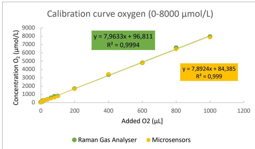
**Figure S5.** Calibration curve for 0 – 1000 µL of oxygen added to an Ar-flushed 4.9 mL glass vial.
