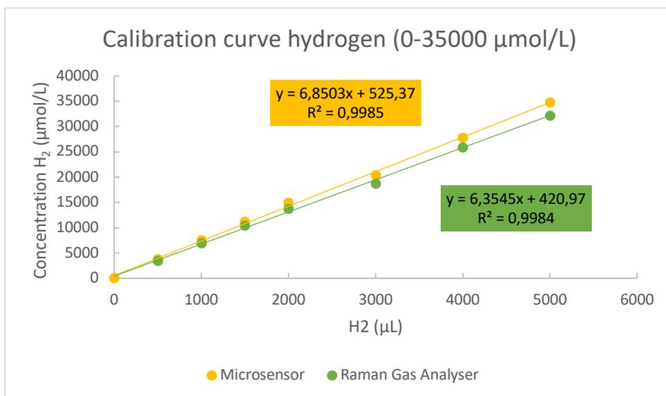
**Figure S4.** Calibration curve for 0 – 5000 μL of hydrogen added to an Ar-flushed 4.9 mL glass vial.
