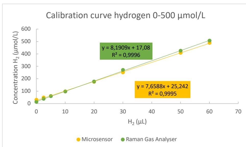
**Figure S1.** Calibration curve for 0 – 60 µL of hydrogen added to an Ar-flushed 4.9 mL glass vial.
