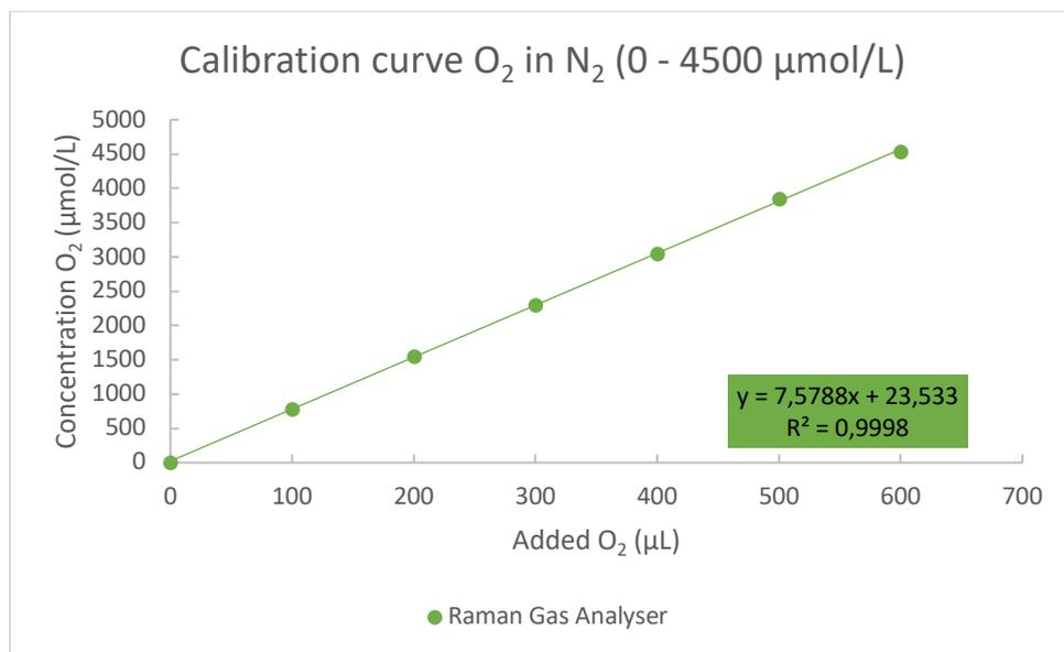
**Figure S7.** Calibration curve for 0 – 600 µL of O<sub>2</sub> added to a N<sub>2</sub>-flushed 4.9 mL glass vial.
