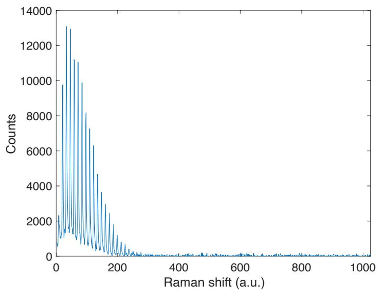
**Figure S9.** Spectral signature of CO recorded with the Raman Gas analyser.
