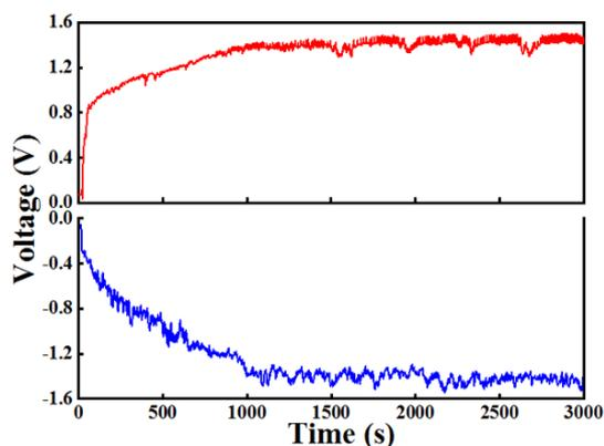
**Fig S7.** The test of exchange positive and negative electrodes to exclude primary battery effect.
