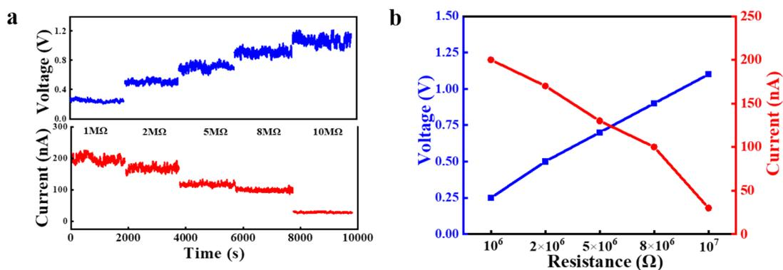
**Fig S8.** (a) The  $V_{oc}$ -t and  $I_{sc}$ -t performance of the NWEs under different external load resistances. (b) Correlation of  $V_{oc}$  and  $I_{sc}$  with applied load resistance.
