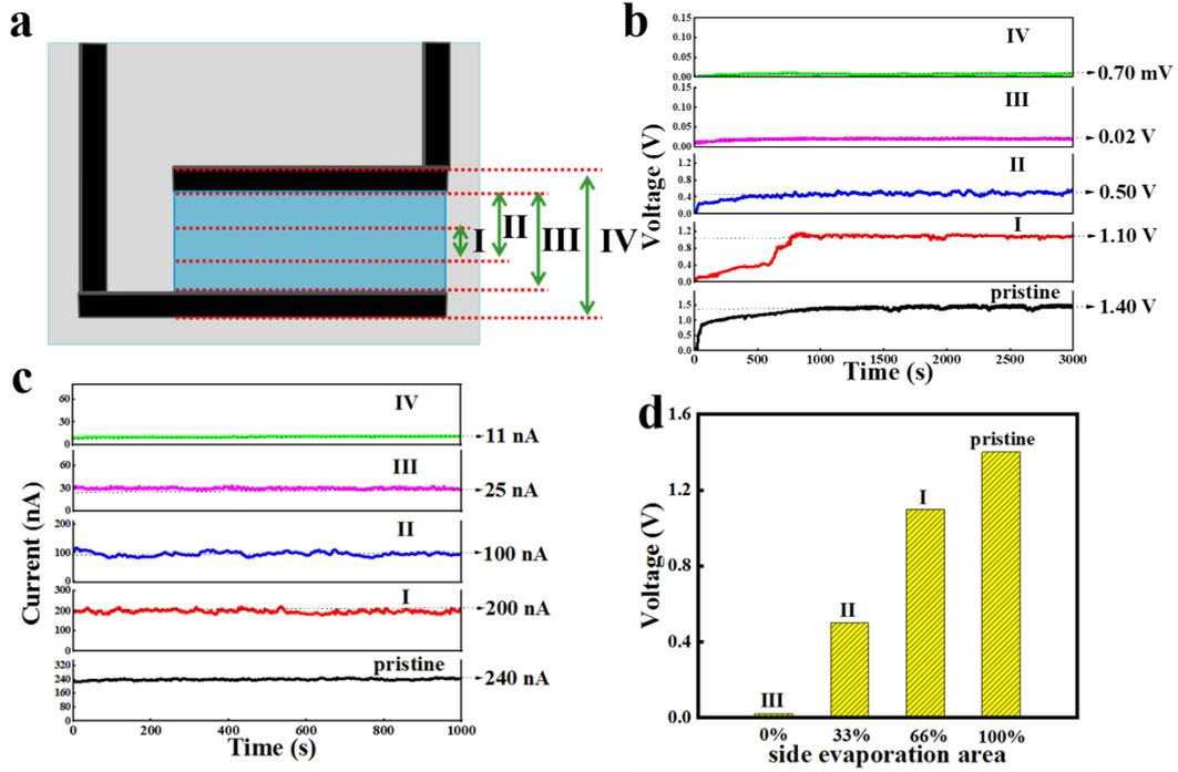
**Fig S4.** (a) Schematic diagram of the side evaporation area with the plastic film and tape to cover the different area. (b) The  $V_{oc}$  of different side evaporation area. (c) The  $I_{sc}$  of different side evaporation area. (d) A histogram of voltage and side evaporation area.
