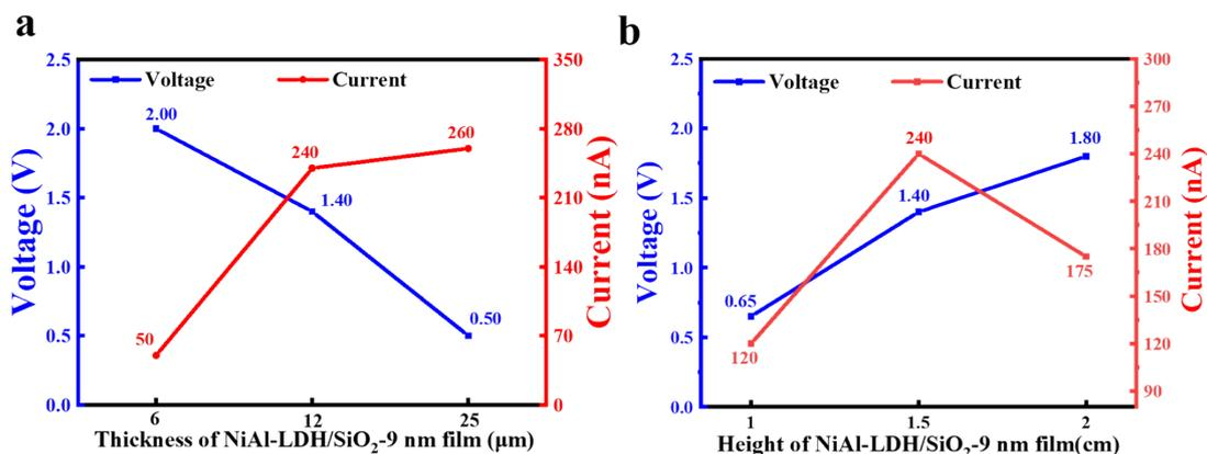
**Fig S5.** The influence of different (a) heights and (b) thicknesses of the NiAl-LDH/SiO<sub>2</sub>-9 nm films on the voltage and current.
