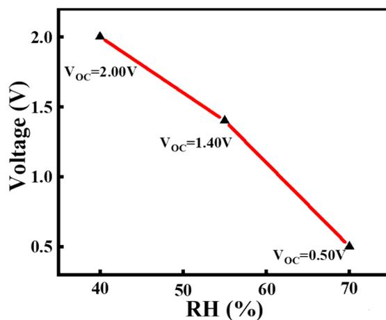
**Fig S6.**  $V_{oc}$  of the NWEGs under different humidity.
