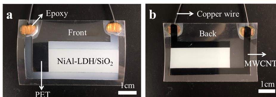
**Fig S1.** The assembly of NiAl- LDH/SiO<sub>2</sub> based NWEG.
