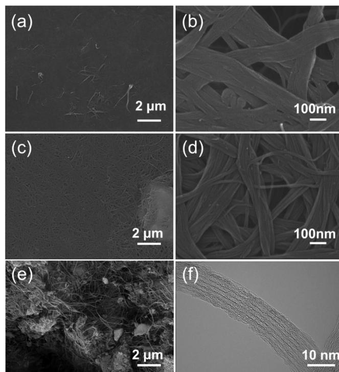
Figure S1. The typical SEM images of (a and b) P-DMF-0.5CNT, (c and d) P-DMF-0.9CNT and (e) EtOH-0.1CNT. (f) The typical TEM image of SWCNT.
