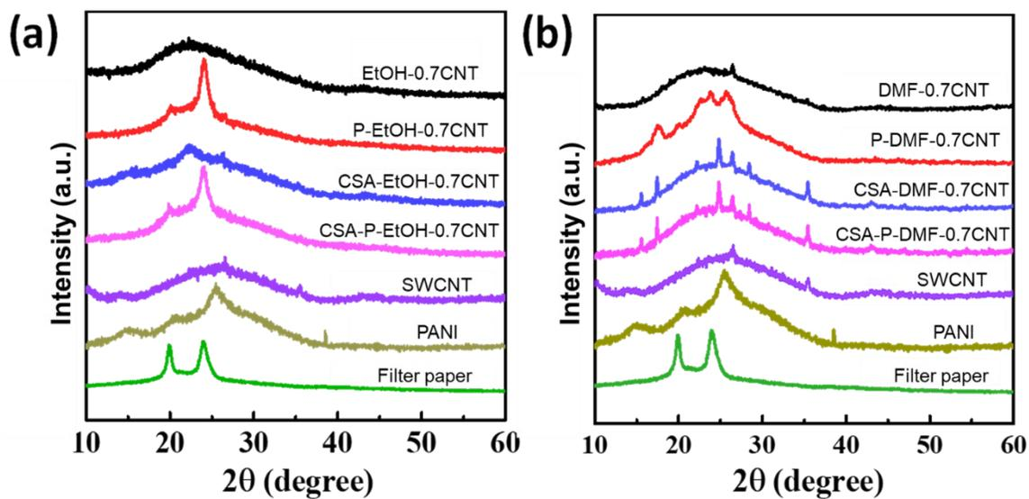
Figure S2. XRD patterns of SWCNT, PANI, filter paper, EtOH-0.7CNT, and DMF-0.7CNT, where CSA- means the sample was prepared from CSA-doped PANI.
