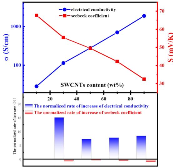
Figure S6. Electrical conductivity ( $\sigma$ ) and Seebeck coefficient ( $S$ ) of P-DMF-xCNT composites with different CNTs content, and the normalized rate of increase of electrical conductivity and Seebeck coefficient.
