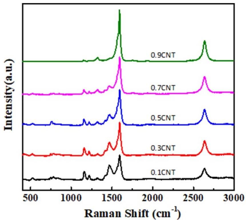
Figure S3. The Raman spectra of P-DMF-xCNT composite films with different CNTs contents (All spectra are normalized).
