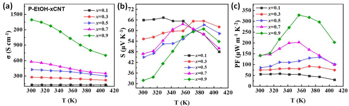
Figure S7. Temperature dependence of (a) electrical conductivity, (b) Seebeck coefficient, and (c) power factor for the P-EtOH-xCNT composite film.
