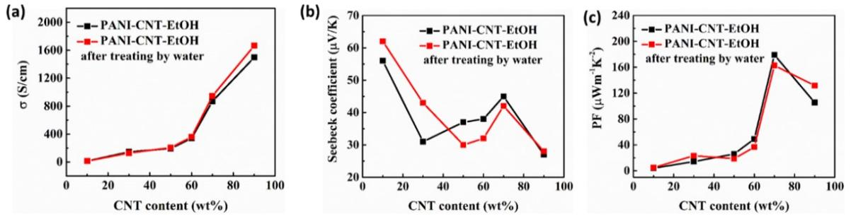
Figure S5. (a) The Seebeck coefficient, (b) conductivity, and (c) power factor of P-EtOH-xCNT with different CNTs content before and after treating by water at room temperature.
