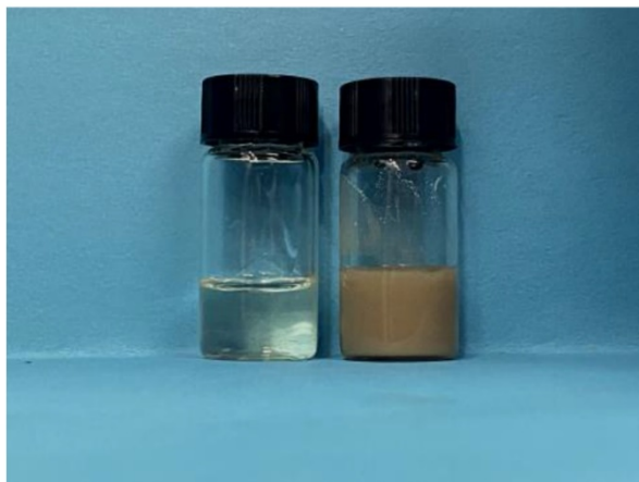
Fig. S2 Photograph of PVDF-Li slurry (left) and PVDF-Li-LZ slurry (right).
