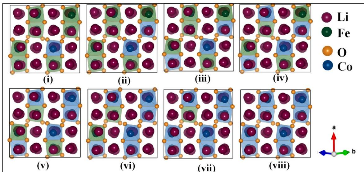
**Figure S2 (b):** The  $\text{Co}^{3+}$  substitution at different Co concentrations in  $\text{Li}_y\text{Fe}_{(1-x)}\text{Co}_x\text{O}_4$ . The Li concentration did not change since we are replacing Fe having +3 oxidation state with Co. The  $\text{FeO}_4$  and  $\text{CoO}_4$  tetrahedra are given in polyhedral representation. The concentration of Co atom increases
