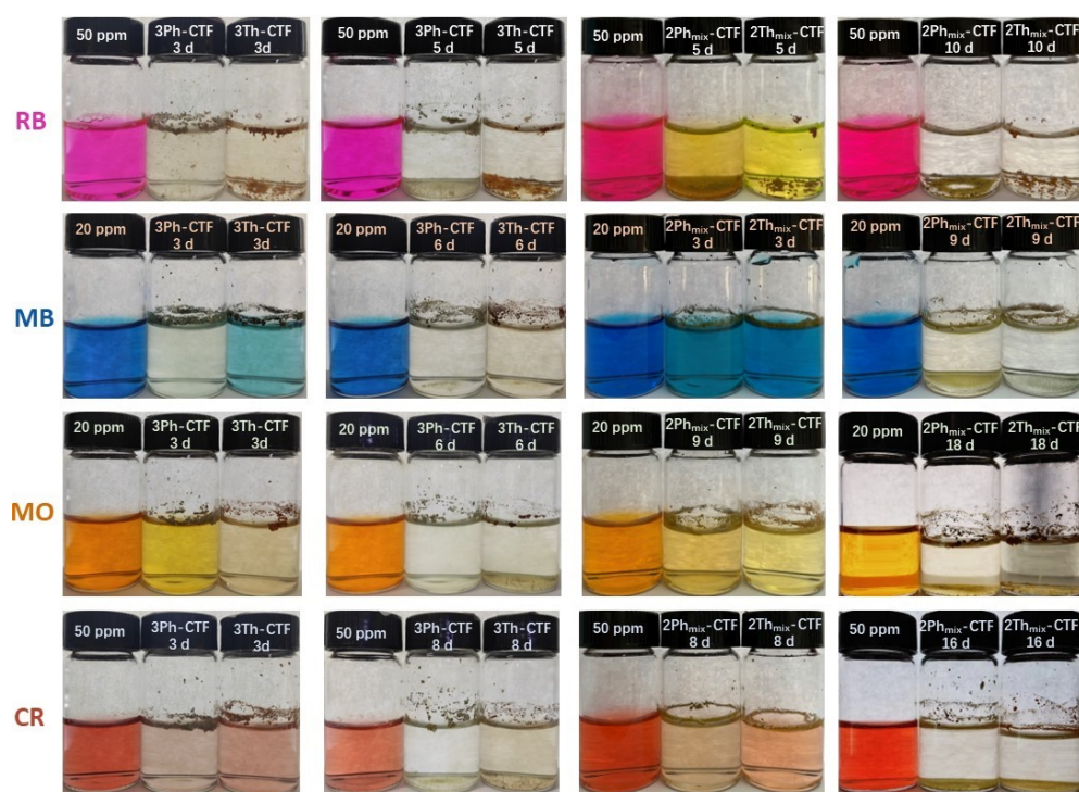
Fig. S8. Photographs of the changes of a) RB b) MB c) MO and d) CR solutions with time in the presence of 3Ph-CTF, 3Th-CTF, 2Ph mix -CTF, and 2Th mix -CTF outside under natural light (standstill state).
