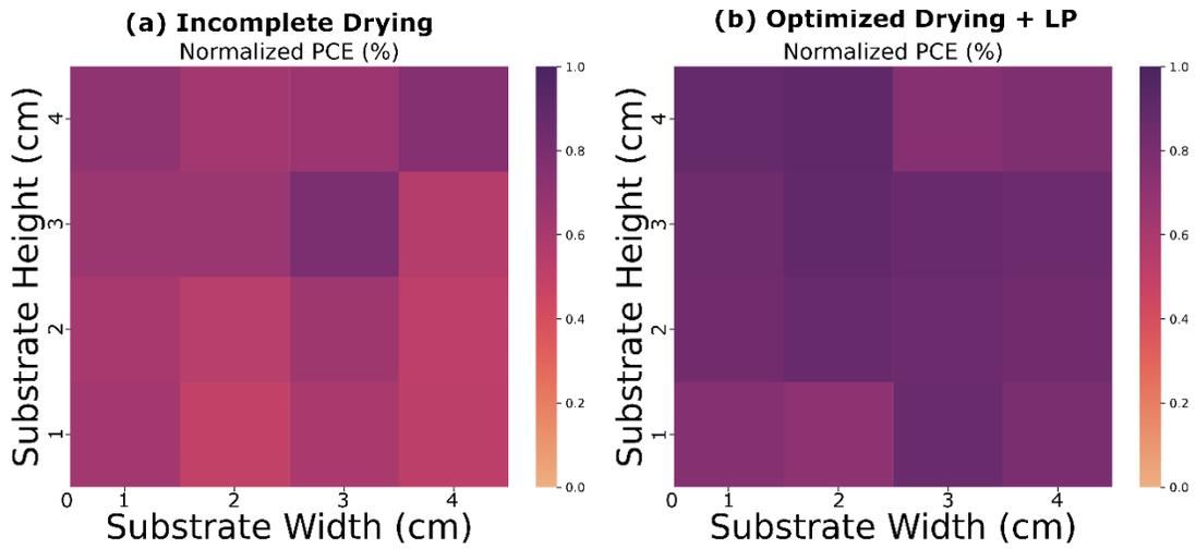
**Figure S6-** The mean normalized distribution of PCE across blade-coated substrates for incomplete and optimized drying.
