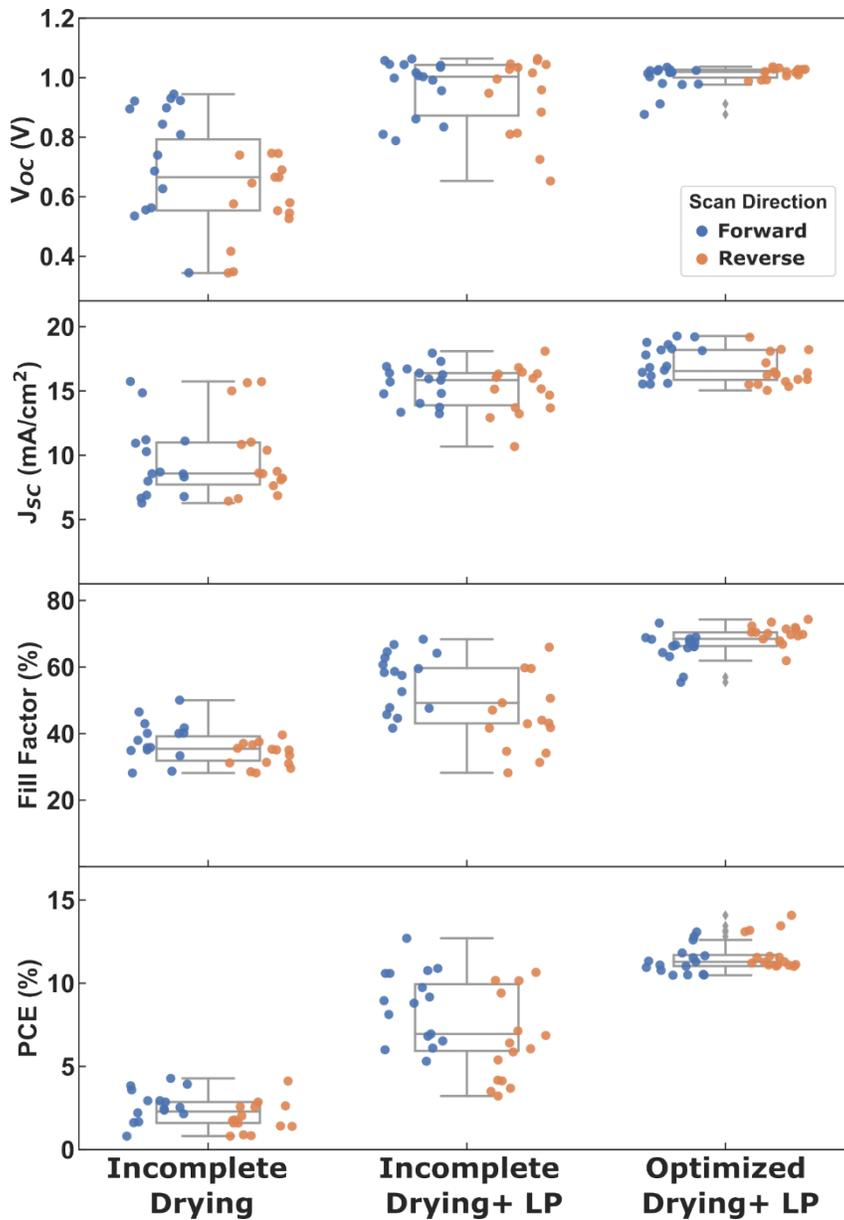
**Figure S5-** PV parameters of blade-coated flexible perovskite solar cells containing 16 cells obtained from one  $5 \times 7$  cm<sup>2</sup> substrate in three conditions: incomplete drying, incomplete drying + LP, and optimized drying + LP.
