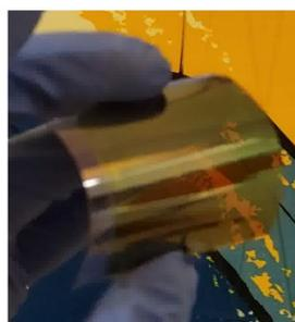
**Figure S2.** Photographs of  $\text{PbI}_2\text{-(FAI)}_{0.3}\text{-(Csl)}_{0.15}$  films blade coated in Ambient dried (a) and Over-dried (b) conditions. (c-d) Photographs of both  $\text{PbI}_2\text{-(FAI)}_{0.3}\text{-(Csl)}_{0.15}$  films and converted perovskite films when the first step is incompletely dried and optimized dried while blading respectively.
