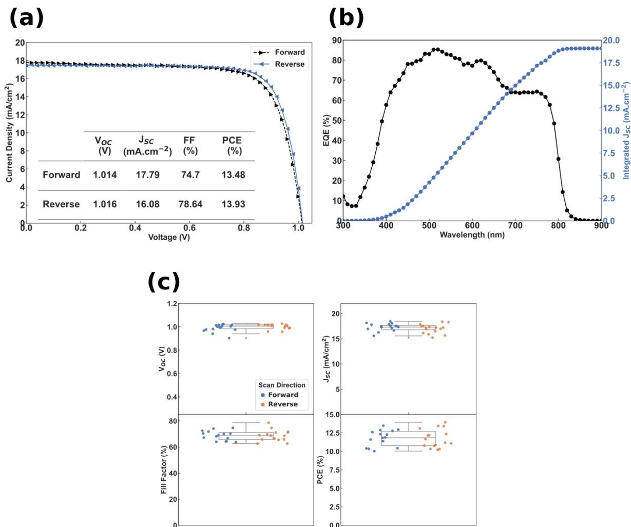
**Figure S7-** (a-b) JV Curve and external quantum efficiency of the champion all-bladed cell. (c) The box plots of PV parameters for all-bladed perovskite solar cells.
