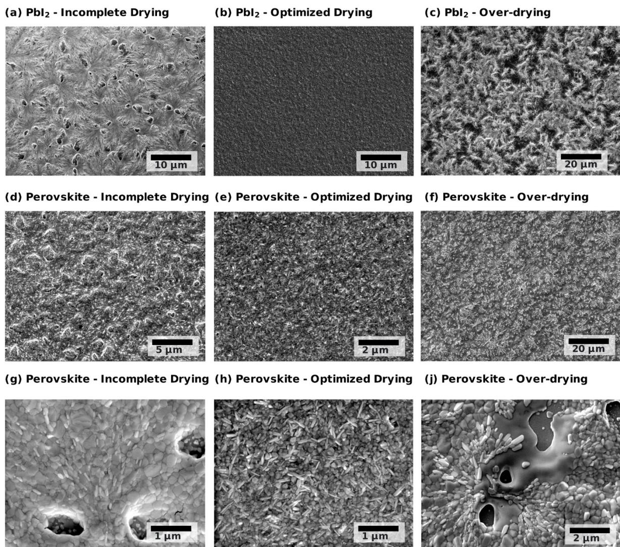
**Figure S3.** SEM images of blade-coated  $\text{PbI}_2\text{-(FAI)}_{0.3}\text{-(Csl)}_{0.15}$  (a-c) and their corresponding double cation perovskite layer (d-j) deposited with three different drying conditions of incomplete drying, optimized drying, and over-drying.
