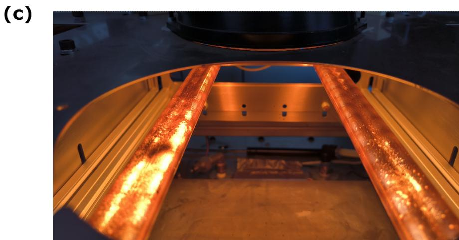
**Figure S1-** (a) The blade coating machine (Charon by Cicci Research). (b) The blade and air nozzle. (c) The IR drying system using Helios Quartz IR Lamps.
