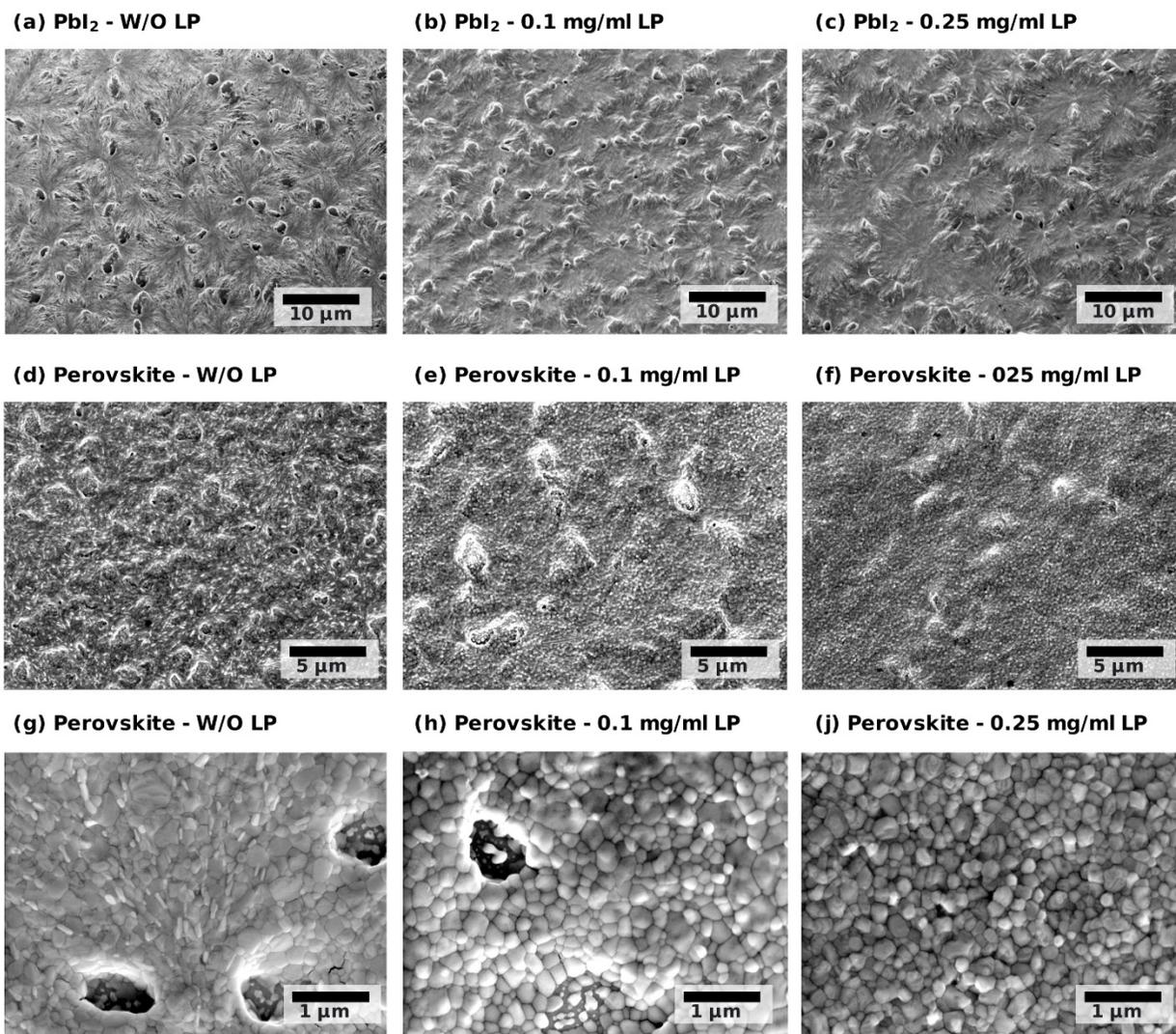
**Figure S4.** SEM images of blade-coated  $\text{PbI}_2$ - $(\text{FAI})_{0.3}$ - $(\text{CsI})_{0.15}$  (a-c) and their corresponding double cation perovskite layer (d-f) deposited with incomplete drying condition without LP additive, with 0.1 mg/ml LP, and with 0.25 mg/ml LP respectively.
