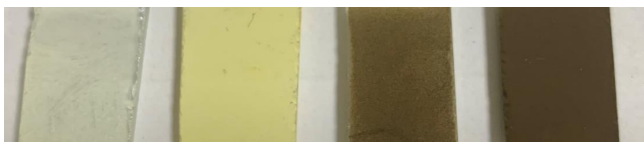
Fig. S9: Pristine, CN-400-air, CN-500-N 2 and CN-500-air samples coated over the FTO (left to right)
