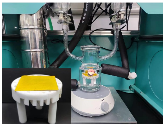
Fig. S9 A photograph of the photocatalytic reaction setup, and inset shows a photograph of the custom-made Teflon sample holder to hold the photocatalyst sheet for photocatalytic reaction.
