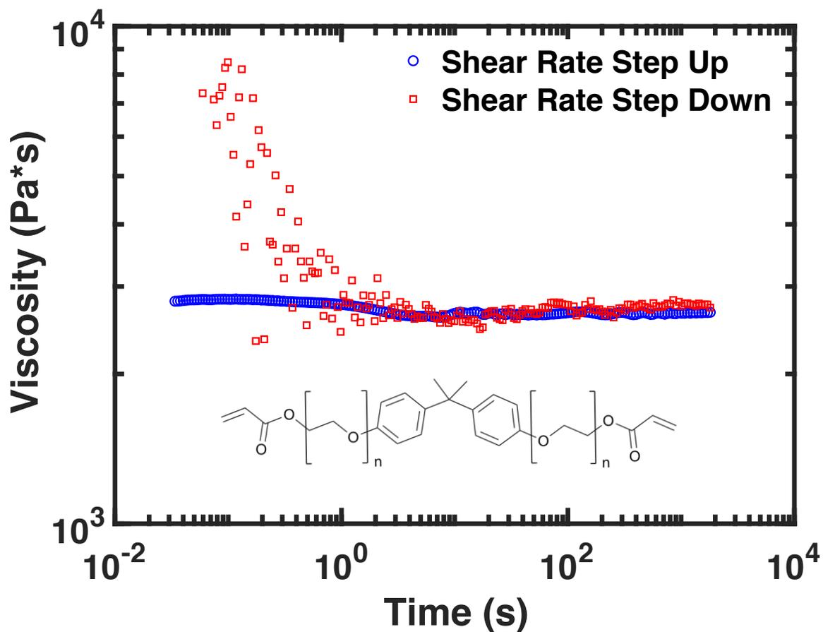
**Figure S4.** Shear rate step-up/step-down test performed on an ink prepared with a non-liquid crystalline diacrylate in place of RM82. As evidenced by the lack of pronounced thinning after the shear rate step-up (performed at  $10 \text{ s}^{-1}$  shear rate) and increasing viscosity after the shear rate step-down, the effects seen in this paper are related to the liquid crystalline nature of the ink used.
