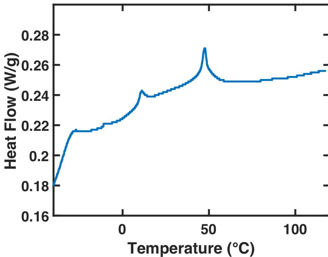
**Figure S3.** Differential Scanning Calorimetry data for the ink used in this study. The second endothermic peak, which occurs at approximately 50 °C, is indicative of the ink's nematic-isotropic transition temperature ( $T_{NI}$ ).
