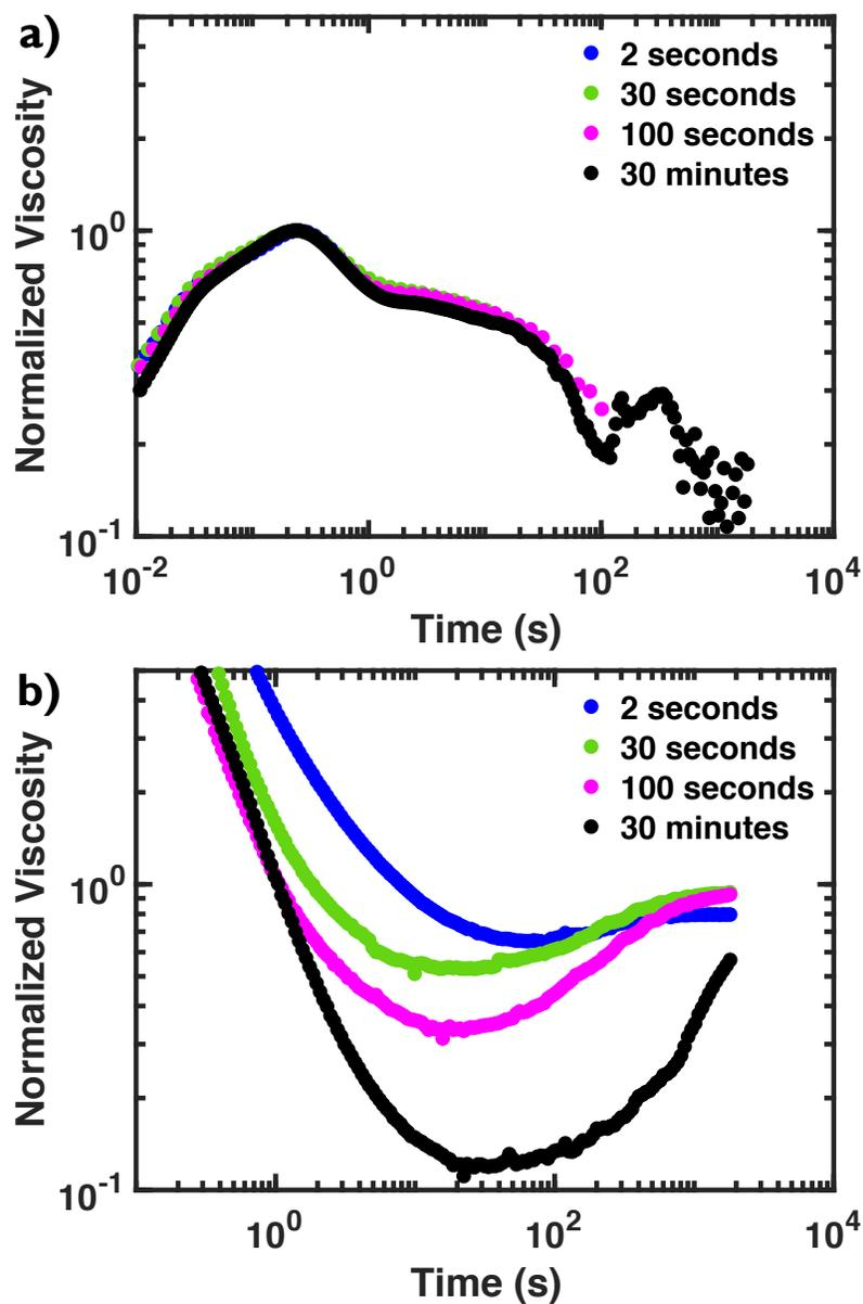
**Figure S6.** (a) Inks after being subjected to a shear rate step-up to  $10 \text{ s}^{-1}$ . This shear rate was then maintained for various times. It can be seen that the data overlay on top of each other well, indicating a degree of replicability. (b) The inks from (a) after being subjected to a shear rate step-down to  $0.01 \text{ s}^{-1}$ . The inks sheared for longer times show smaller minimum viscosities, which correlates with better liquid crystalline alignment.
