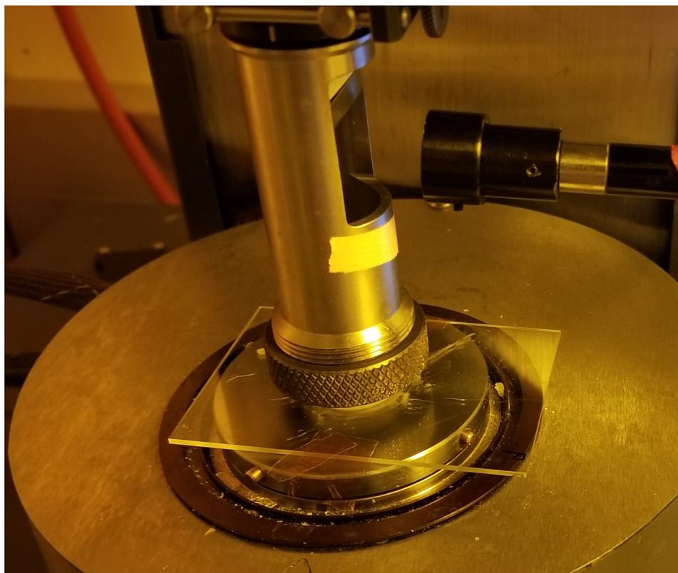
**Figure S1.** Picture of the UV curing rheometer setup. A glass slide is attached to the bottom rheometer plate with Kapton tape. After shearing and curing the glass slide and rheometer head can each be removed from the machine, allowing for polarized microscopy of the LCE.
