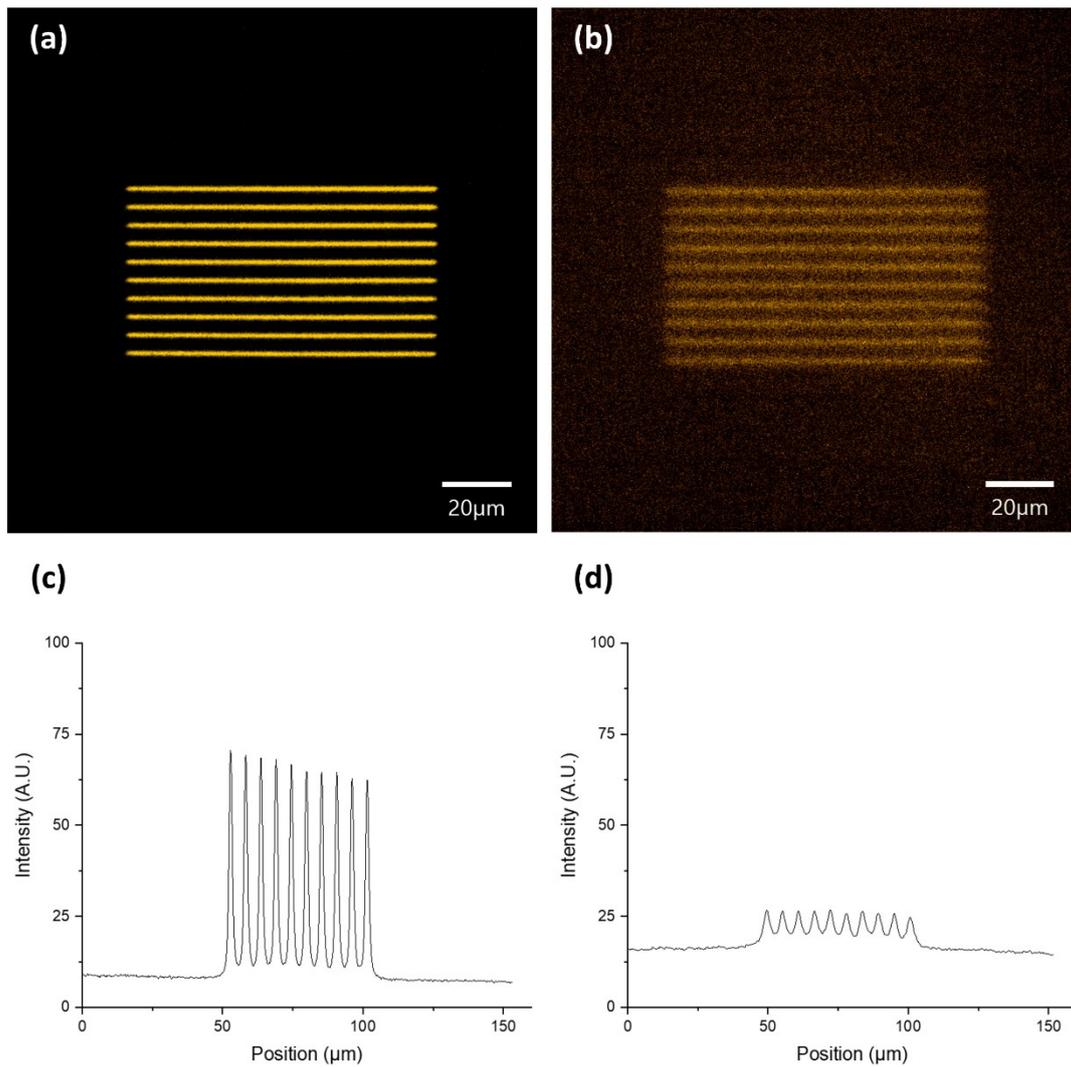
**Fig. S4** Fluorescence images of patterning on the PAAm-sodium acrylate hydrogel with different incubation solutions. (a) Image obtained from patterning using CF-633 NHS ester as incubation solution and 640 nm laser for exposure. (b) Image obtained from patterning using Alexa Fluor 546 carboxylic acid, succinimidyl ester as incubation solution and 561 nm laser for exposure. (c) Intensity profiles of (a). (d) Intensity profiles of (b).
