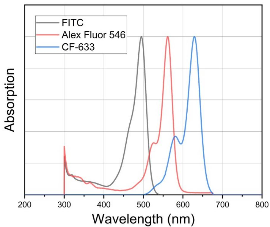
**Fig. S5** Absorbance spectra of the fluorophores used: FITC, Alexa Fluor 546, CF-633.
