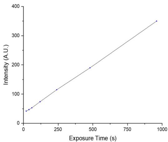
**Fig. S7** Relationship between the fluorescence intensity of the patterns and exposure time. (a) Confocal microscopy images of PAAm-sodium acrylate hydrogels, which were patterned with a 405 nm laser for varying exposure times. (b) Quantitative analysis of the fluorescence intensity versus exposure time.
