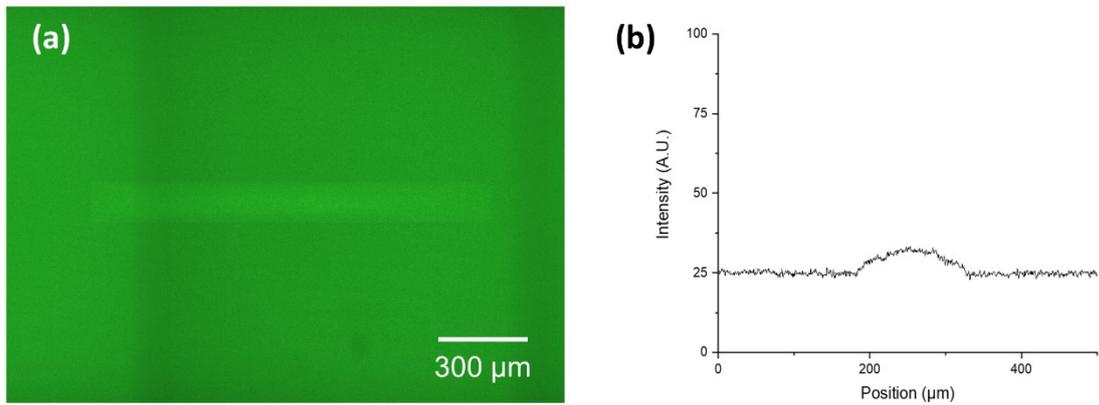
**Fig. S2** Fluorescence image of photobleached fluorescein on the PAAm hydrogel after patterning. (a) Image obtained from patterning using 405 nm laser for exposure. (b) Intensity profiles of (a).
