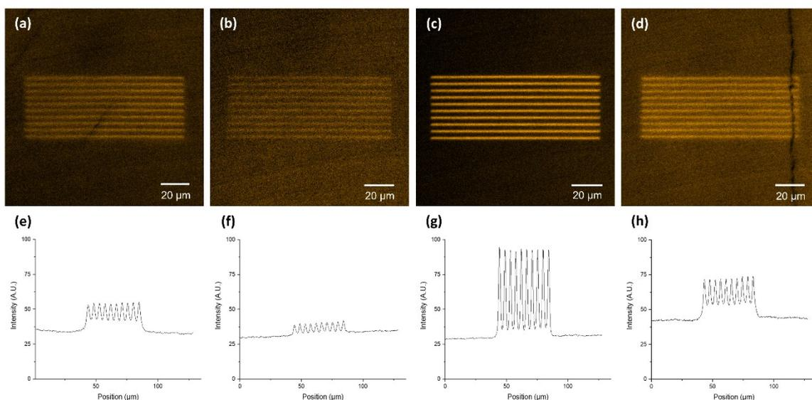
**Fig. S6** Fluorescence images of patterning on the PAAM-sodium acrylate hydrogel using CF-633 NHS ester as incubation solution. (a) 405 nm, (b) 488 nm, (c) 561 nm, (d) 640 nm laser exposed for patterning. (e) Intensity profiles of (a). (f) Intensity profiles of (b). (g) Intensity profiles of (c). (h) Intensity profiles of (d).
