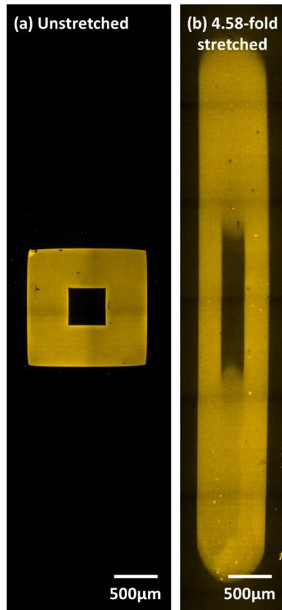
**Fig. S11** Macroscopic patterning for demonstration of the local stretchability control in mm scale. Fluorescence images of patterning using 5-aminoFITC as incubation solution on the PAAm hydrogel with 405 nm laser. (a) Confocal microscopy image obtained before stretching. (b) Confocal microscopy image obtained after 4.58 times stretching.
