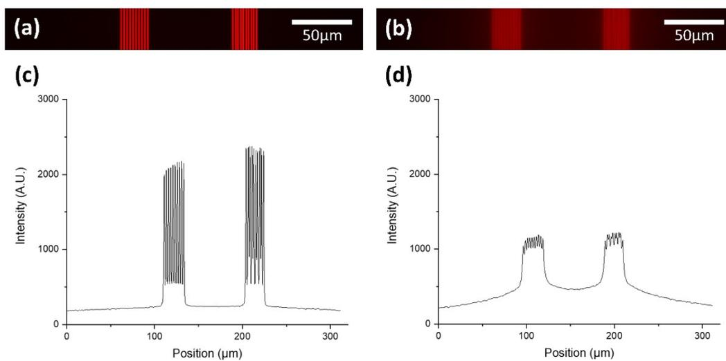
**Fig. S3** Fluorescence images of patterning using 5-aminoFITC as incubation solution on the PAAm hydrogel with different laser wavelengths. (a) Image obtained from patterning using 405 nm laser for exposure. (b) Image obtained from patterning using 488 nm laser for exposure. (c) Intensity profiles of (a). (d) Intensity profiles of (b).
