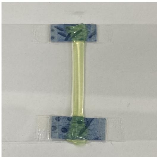
**Fig. S8** Image of stretchable hydrogel mounting in the stretched state.
