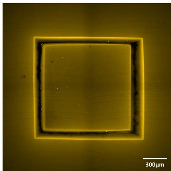
**Fig. S9** Fluorescence image of the ablated hydrogels at an excessive laser power.
