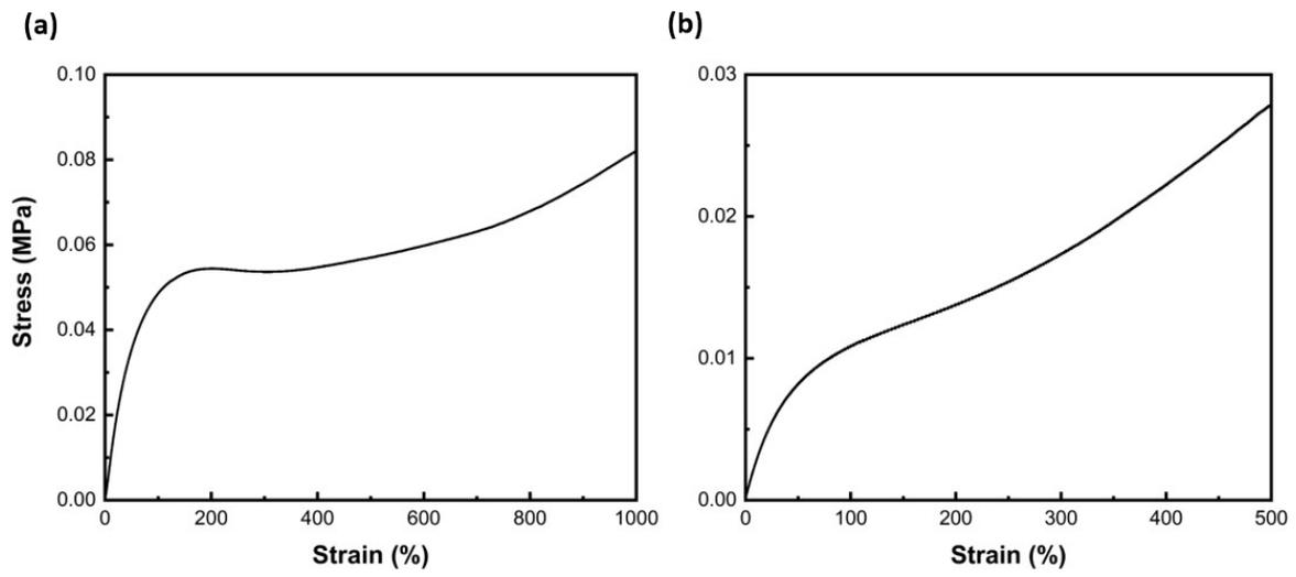
**Fig. S10** Stress-strain curve of the acrylamide hydrogel (a) after synthesis and (b) after immersion in deionized water.
