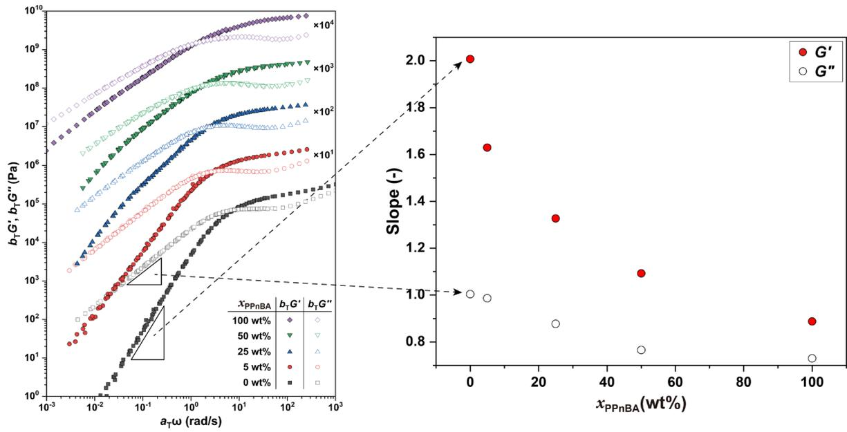
**Figure S8.** Slope of  $G'$  and  $G''$  in the lower frequency range as a function of  $x_{PPnBA}$ . The slopes were obtained by fitting the experimental data with the equation,  $G(T) = a \exp(b\omega)$ .
