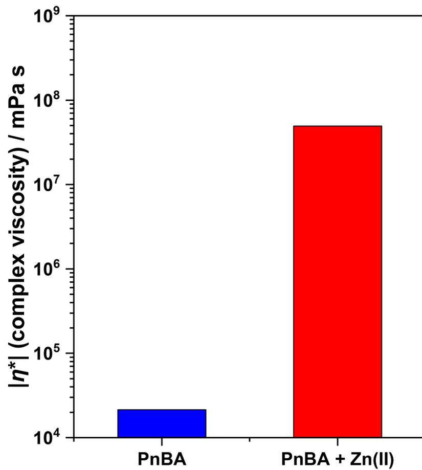
**Figure S4.** Complex viscosities of the PnBA melt and PnBA elastomer crosslinked by Zn(II) at 20 °C.
