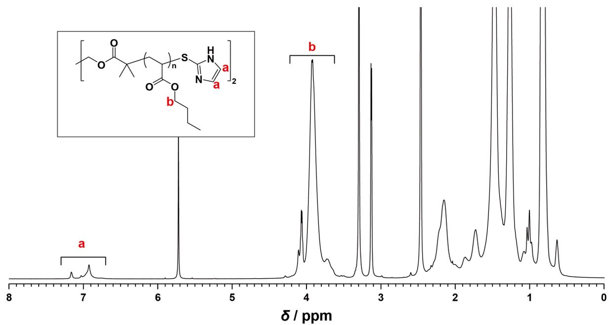
**Figure S2.** <sup>1</sup>H-NMR spectrum of imidazole-functionalized PnBA (imi-PnBA<sub>45</sub>-imi).
