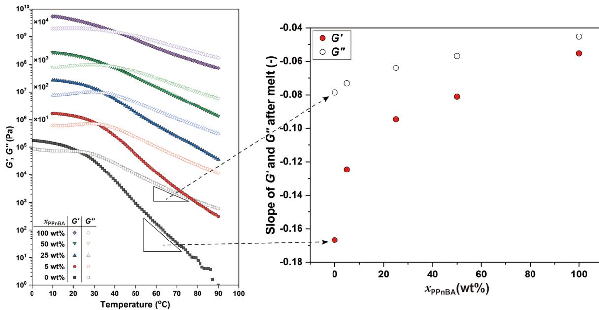
**Figure S7.** Slope of  $G'$  and  $G''$  as a function of  $x_{PPnBA}$  after melting. The slopes were obtained by fitting the experimental data with the equation,  $G(T) = a \exp(bT)$ .
