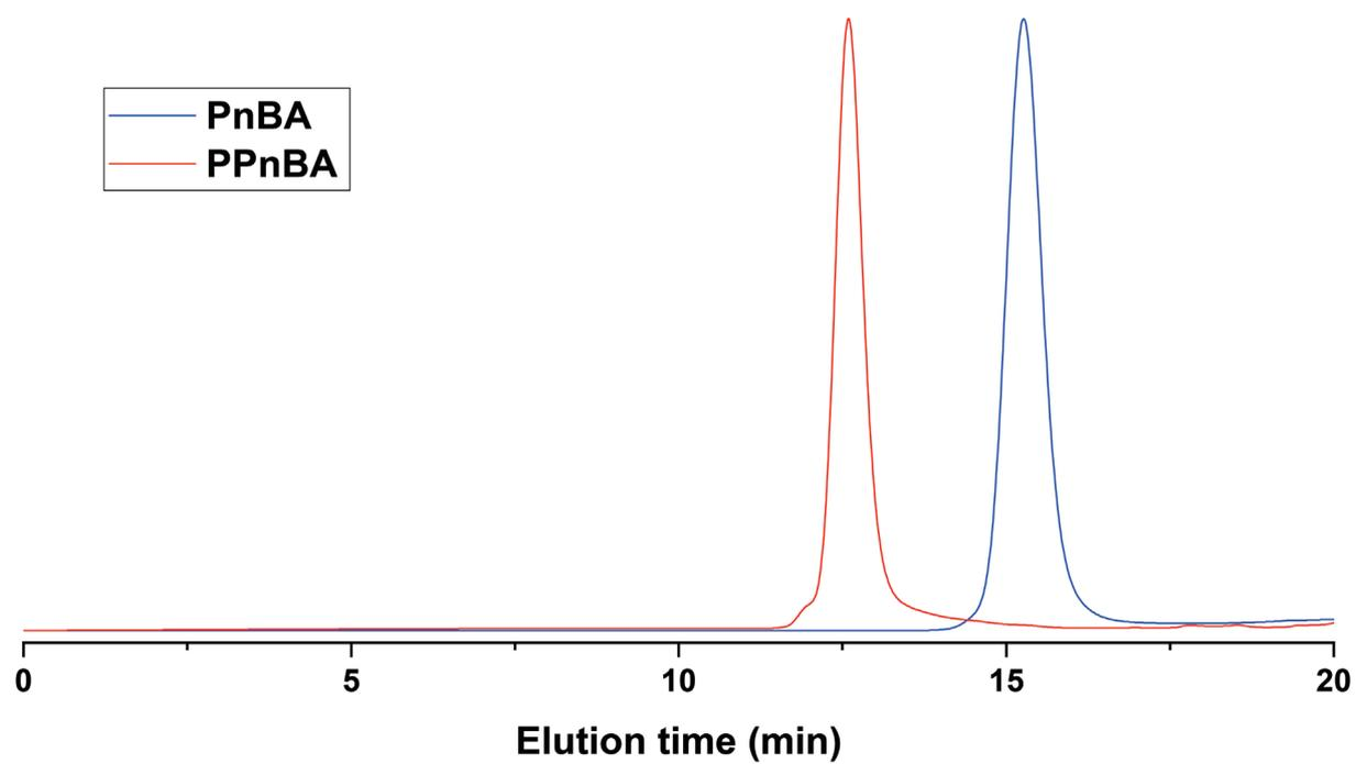
**Figure S1.** GPC traces of imidazole-functionalized PnBA (imi-PnBA<sub>45</sub>-imi) and PPnBA (P(PnBA<sub>41</sub>-imi)<sub>50</sub>) synthesized in this study.
