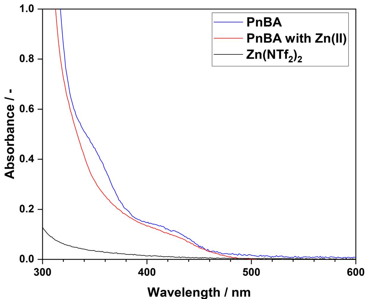
**Figure S5.** UV-Vis spectra of PnBA and PnBA added with Zn(II) and Zn(NTf<sub>2</sub>)<sub>2</sub> in acetonitrile. The polymer concentrations were fixed at 0.2 wt%.
