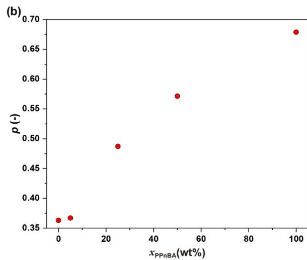
**Figure S10.** Calculated end-group reactivity of the PnBA/PPnBA blended elastomer as a function of  $x_{PPnBA}$ .
