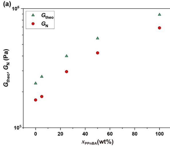
**Figure S9.** Plateau modulus ( $G$ ) as a function of  $x_{\text{PPnBA}}$  for defect-free elastomers. Comparison of the experimentally obtained plateau modulus ( $G_{\text{N}}$ ) with the theoretically calculated plateau modulus ( $G_{\text{theo}}$ ).
