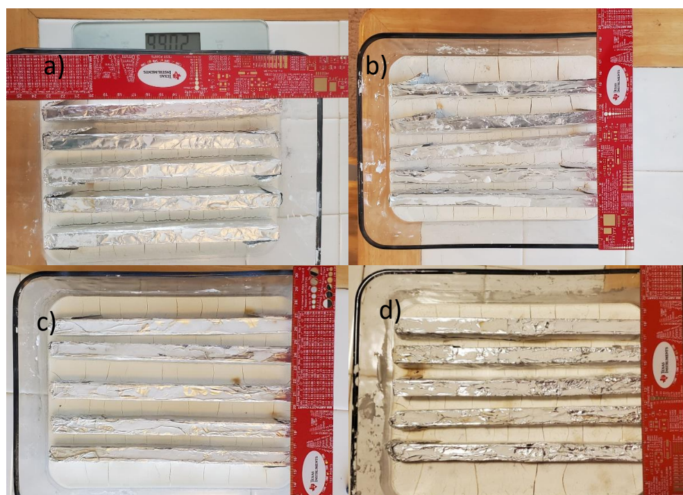
Figure 1: Corn starch cakes formed in wooden troughs. (a) Experiment conducted with lamp at 13 cm from dish. (b) Experiment conducted with lamp at 40 cm from dish. (c) Experiment conducted with lamp at 20 cm from dish (d) Experiment conducted without lamp.
