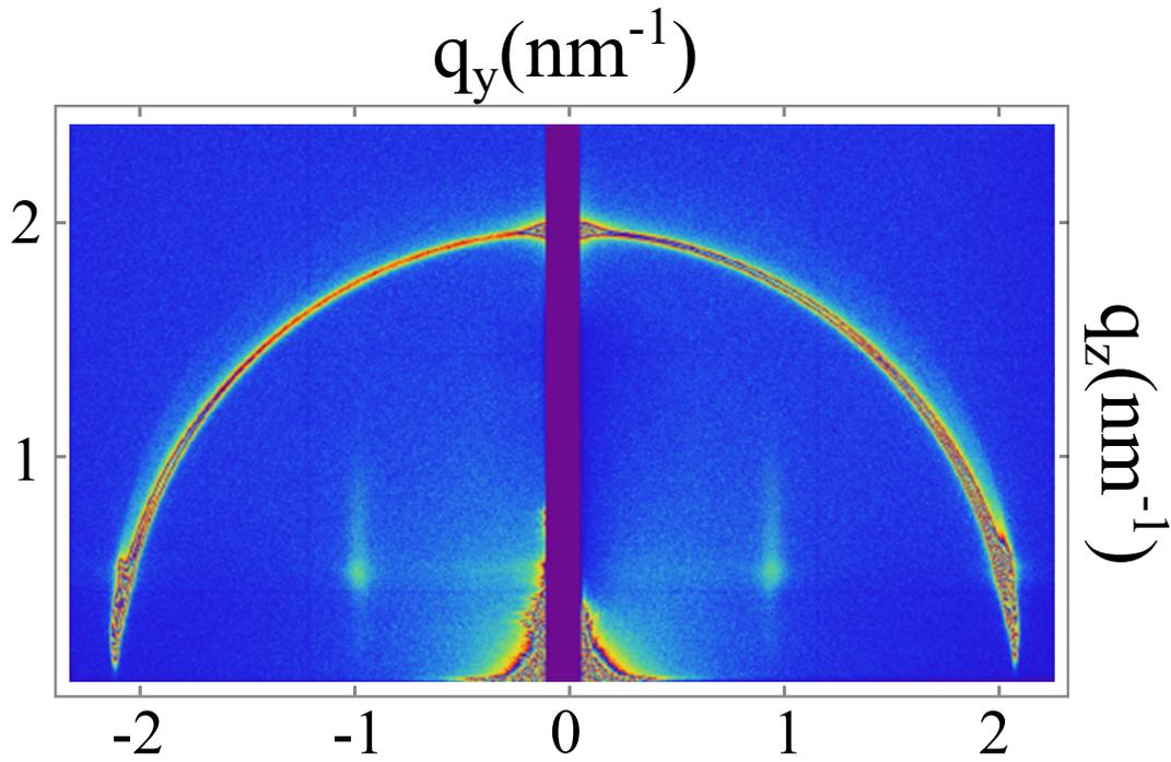
Fig.SI 5 GISAXS scattering pattern of DRs composite sample zone dominated by oily streaks ( $e = 170$  nm,  $C_{avg} = 980$  DRs  $\mu\text{m}^{-2}$ ), where the X-ray beam is parallel to the substrate (incident angle  $0.25^\circ$ ). The half-circle corresponds to the LC smectic layers and the scattering rods at  $q_y = \pm 0.9$   $\text{nm}^{-1}$  are in agreement with a side-by-side packing of DRs in oily streaks with a center-to-center distance of 8.06 nm between DRs.
