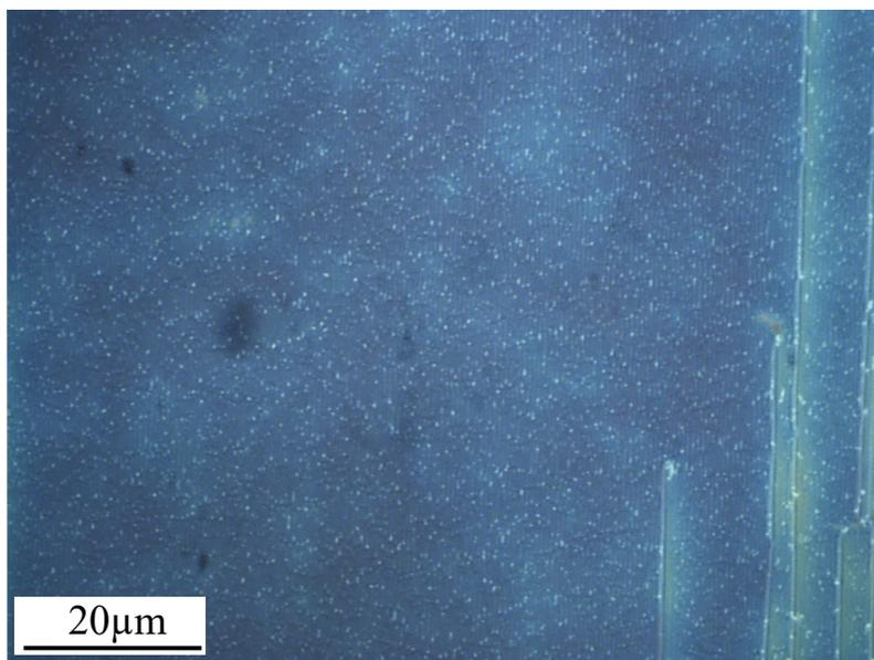
Fig.SI 3 POM picture with parallel polarizers of a 8CB film with low concentration ( $l_{avg} = 120$  nm and GNP concentration  $C_{avg} = 1700$  GNPs  $\mu\text{m}^{-2}$ ). Only small ribbons are observed, suggesting that the area is mostly covered by GNP chains confined in the 1D defects<sup>4</sup>.
