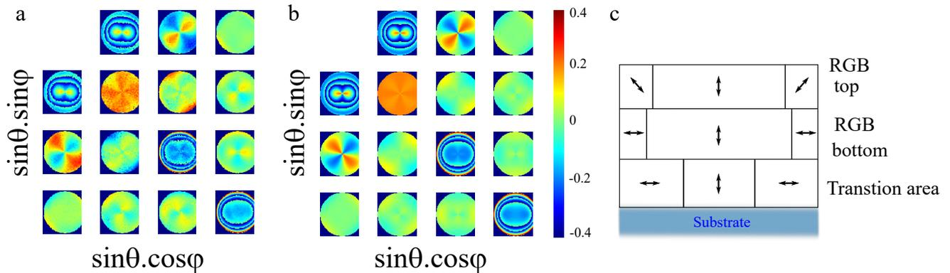
Fig.SI 1 (a) Measured and (b) calculated Mueller matrix elements for a 8CB film of 180 nm average thickness, containing large stripes (as mapped by the objective ( $x = \sin\theta \cdot \cos\phi, y = \sin\theta \cdot \sin\phi$ )). (c) The corresponding simplified model of the LC hemicylinders shown in side view with domains of constant optic axes directions indicated by the double arrows.
