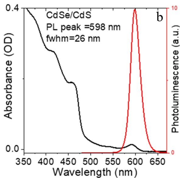
Fig.SI 4 (a) Transmission Electron Microscopy (TEM) of CdSe/CdS dot-in-rods (diameter 7 nm and length 22 nm) drop casted directly on a copper TEM grid, using a JEOL 2010 microscope operated at 200 kV. (b) The corresponding absorption and photoluminescence (PL) spectrum with a PL peak at 598 nm.
