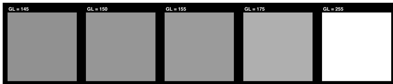
Fig. S1: Digital photomasks employed for the fabrication of the homogeneous gel samples with  $GL = \{145, 150, 155, 175, 255\}$ .
