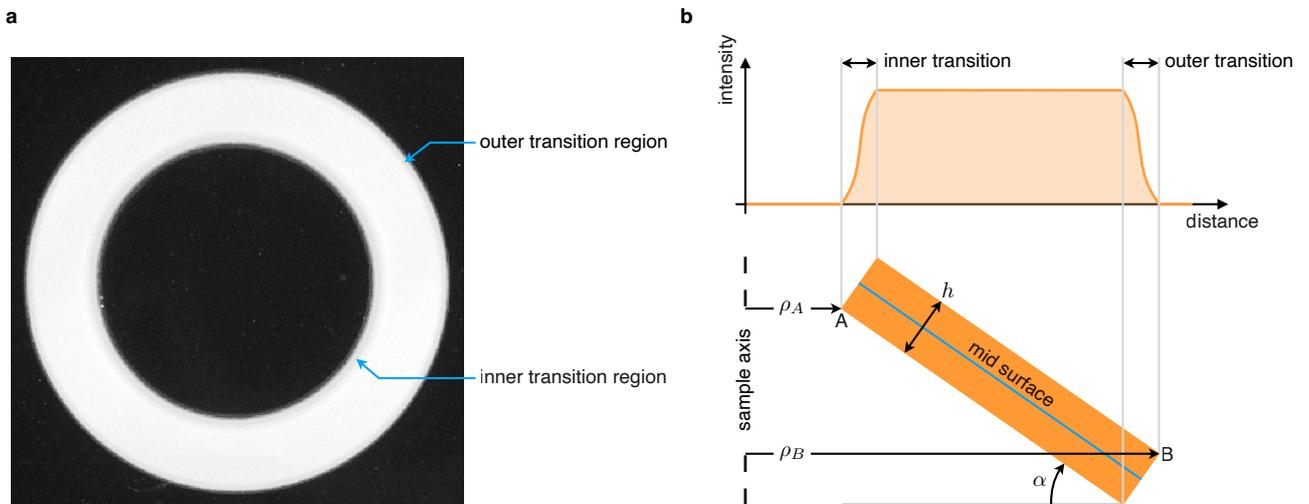
Fig. S3: (a) Typical top view of a gel sample with indication of the inner and outer transition regions in the image and (b) a graphical description of the effect of the gel samples edges on the image intensity profile.
