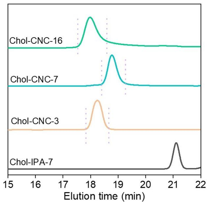
**Fig. S19** GPC traces of the Chol-IPA-7 and Chol-CNCs, the polymer dispersity indexes (PDI) of the molecular weights are evaluated to be 1.03, 1.02 and 1.05 for Chol-CNC-3, Chol-CNC-7, and Chol-CNC-16, respectively.
