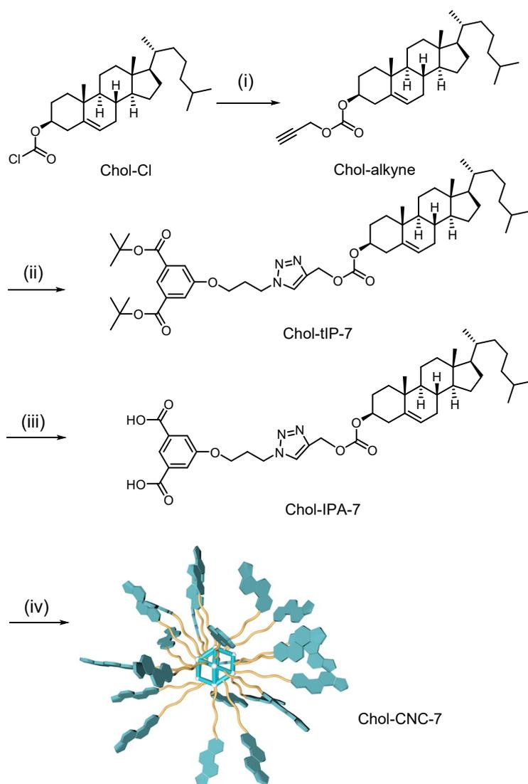
**Scheme S2.** Reaction conditions: (i) propargyl alcohol, DMAP, TEA, CH<sub>2</sub>Cl<sub>2</sub>, RT; (ii) tIP-N<sub>3</sub>, CuBr, PMDETA, toluene, RT; (iii) TFA, CH<sub>2</sub>Cl<sub>2</sub>, RT; (iv) Cu (CH<sub>3</sub>CO<sub>2</sub>)<sub>2</sub>·H<sub>2</sub>O, DMF, THF, RT.
