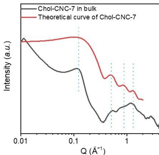
**Fig. S32** SAXS patterns of bulk Chol-CNC-7 and theoretical curve of Chol-CNC-7.
