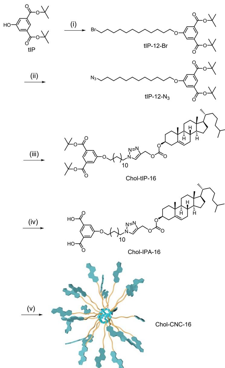
**Scheme S3.** Reaction conditions: (i) 1,12-dibromododecane, K<sub>2</sub>CO<sub>3</sub>, KI, acetone, 80 °C; (ii) NaN<sub>3</sub>, DMF, 80 °C; (iii) CuBr, PMDETA, toluene, RT; (iv) TFA, CH<sub>2</sub>Cl<sub>2</sub>, RT; (v) Cu (CH<sub>3</sub>CO<sub>2</sub>)<sub>2</sub>·H<sub>2</sub>O, DMF, THF, RT.
