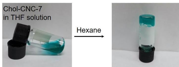
**Fig. S23** Photographs of supramolecular gel of Chol-CNC-7 in THF/hexane (20.0 mg Chol-CNC-7, hexane (0.2 mL)/THF (0.2 mL)).
