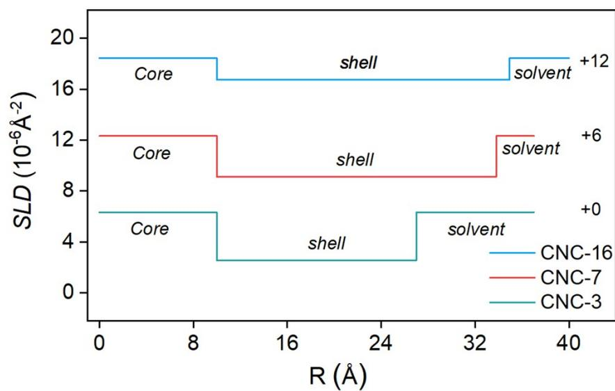
**Fig. S20** The fitted scattering length density (SLD) profile of Chol-CNCs arising from the SANS data on the basis of core-shell model, which reflects the contrast of inner core and outer shell character.
