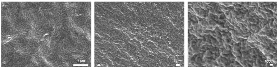
**Fig. S28** SEM images of the freeze-dried Chol-CNC-7 supramolecular gel (160.0 mg Chol-CNC-7, hexane (0.7 mL)/THF (0.8 mL)).
