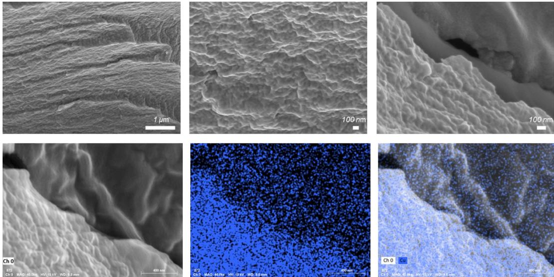
**Fig. S27** SEM and EDX images of the freeze-dried Chol-CNC-3 supramolecular gel (20.0 mg Chol-CNC-3, hexane (0.14 mL)/THF (0.04 mL)) (blue, Cu atom).
