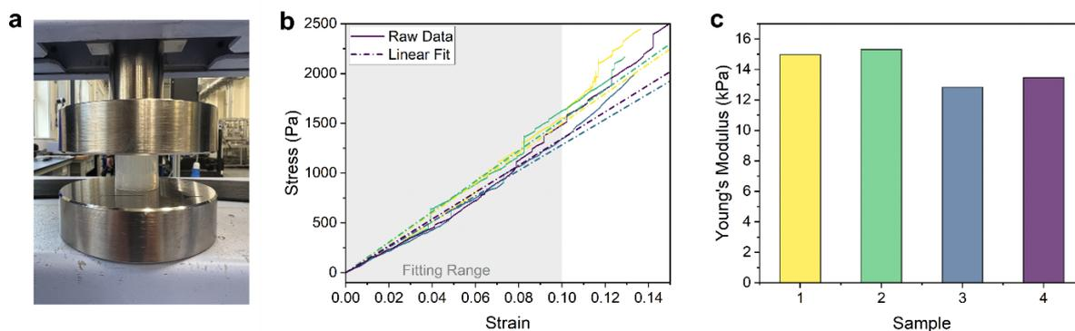
Supplementary Figure 1. Uniaxial compression testing of 7.5% polyacrylamide hydrogels. (a) Experimental setup and sample geometry, (b) linear fits of stress/strain data (to a maximum of 0.1 strain) for four hydrogel samples, and (c) resultant Young's moduli for each sample.
