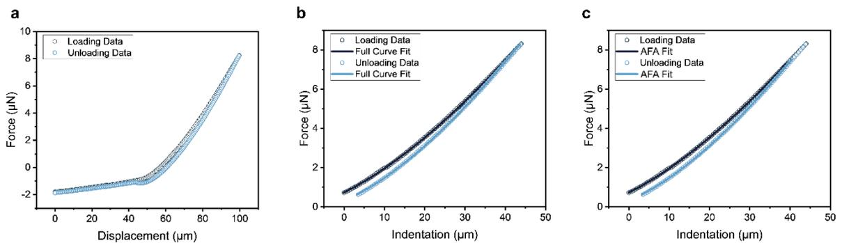
Supplementary Figure 10. Typical data obtained by indentation of 5% polyacrylamide hydrogels. (a) Raw force-displacement data, and processed data with (b) full curve fitting and (c) AFA fitting.
