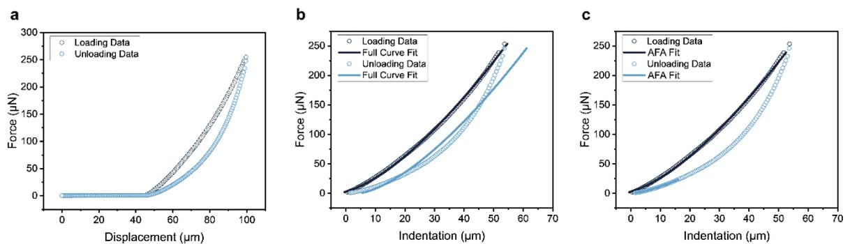
Supplementary Figure 6. Typical data obtained by indentation of 2% agarose hydrogels. (a) Raw force-displacement data, and processed data with (b) full curve fitting and (c) AFA fitting.
