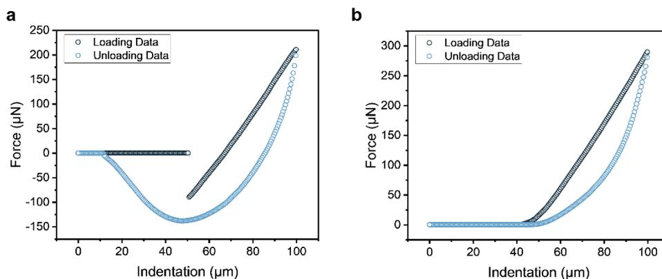
Supplementary Figure 2. Typical load-displacement curves obtained by the indentation of 2% agarose hydrogels in air (a), and with aqueous medium covering the sample (b).
