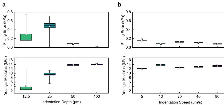
Supplementary Figure 4. Box charts showing Young's modulus values and associated fitting errors obtained by indenting 10% PEGDA hydrogels with a  $300\ \mu\text{m}$  diameter spherical probe. (a) Effects of altering indentation depth, and (b) effects of altering the indentation speed.
