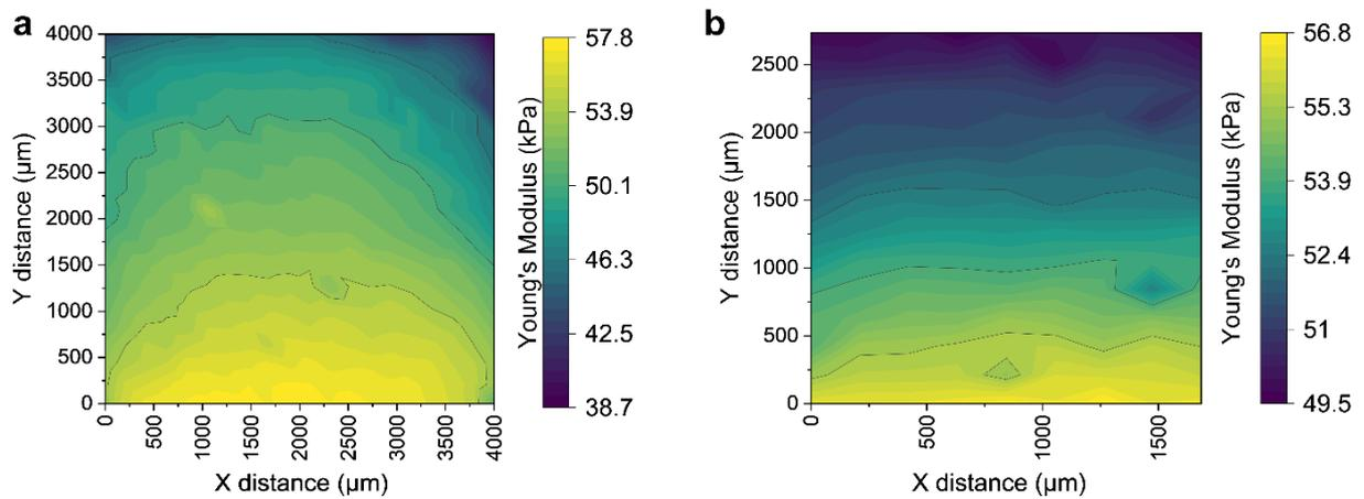
Supplementary Figure 13. (a) Contour plot of a 20x20 array measurement of a PEGDA hydrogel irradiated through a gradient mask. (b) Contour plot of selected region of (a) displaying an approximately linear gradient in Young's modulus along the Y axis.
