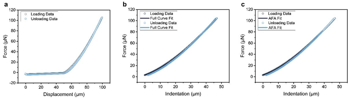
Supplementary Figure 9. Typical data obtained by indentation of 10% PEGDA hydrogels. (a) Raw force-displacement data, and processed data with (b) full curve fitting and (c) AFA fitting.
