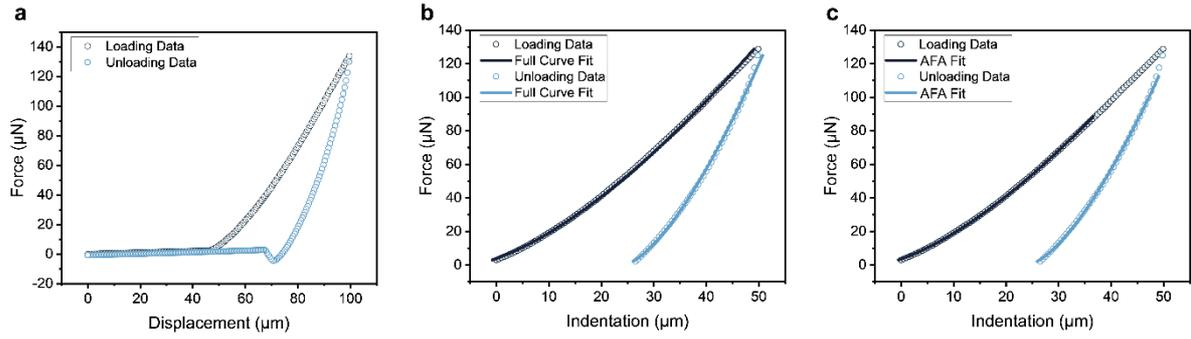
Supplementary Figure 8. Typical data obtained by indentation of 1% alginate hydrogels. (a) Raw force-displacement data, and processed data with (b) full curve fitting and (c) AFA fitting.
