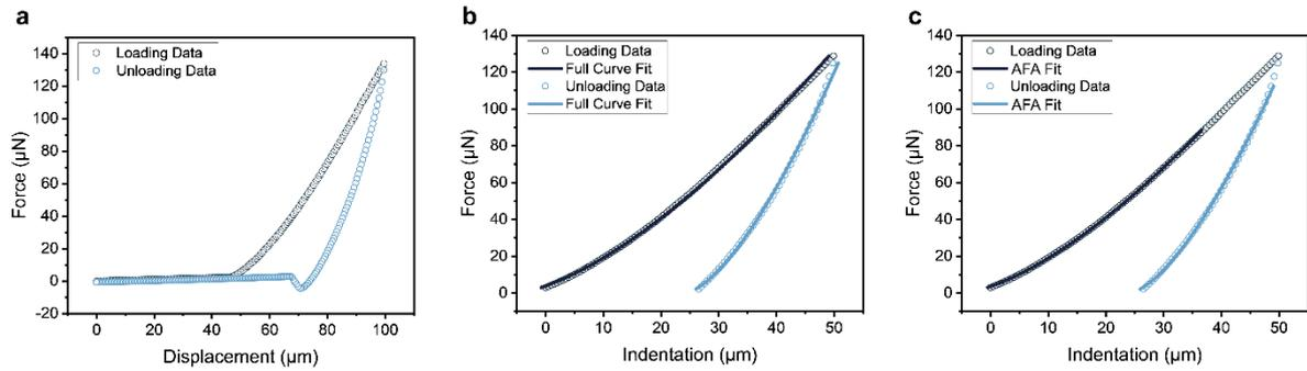
Supplementary Figure 11. Typical data obtained by indentation of 10% polyacrylamide hydrogels. (a) Raw force-displacement data, and processed data with (b) full curve fitting and (c) AFA fitting.
