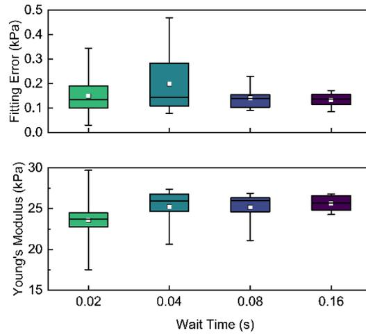
Supplementary Figure 3. Box charts showing Young's modulus values and associated fitting errors obtained by indenting 2% agarose hydrogels to a depth of approximately  $50\ \mu\text{m}$  at a speed of  $10\ \mu\text{m}\ \text{s}^{-1}$  with the stick-slip actuator whilst varying the wait time between actuation steps.
