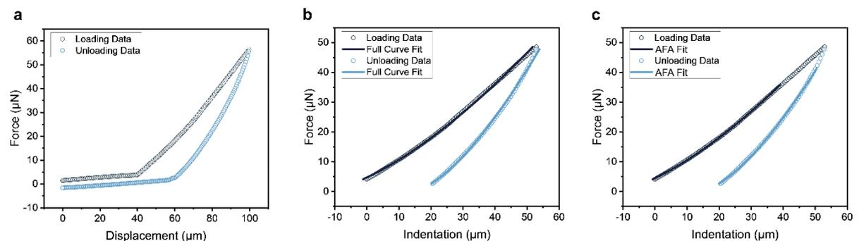
Supplementary Figure 7. Typical data obtained by indentation of 0.5% alginate hydrogels. (a) Raw force-displacement data, and processed data with (b) full curve fitting and (c) AFA fitting.
