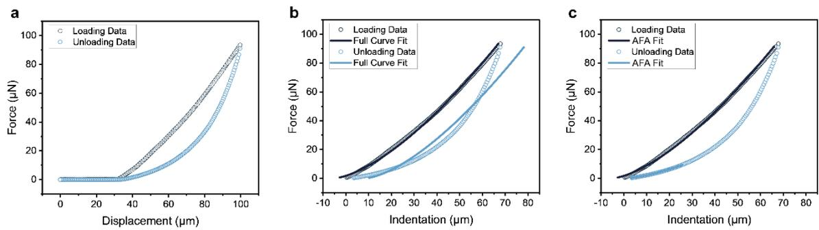
Supplementary Figure 5. Typical data obtained by indentation of 1% agarose hydrogels. (a) Raw force-displacement data, and processed data with (b) full curve fitting and (c) AFA fitting.
