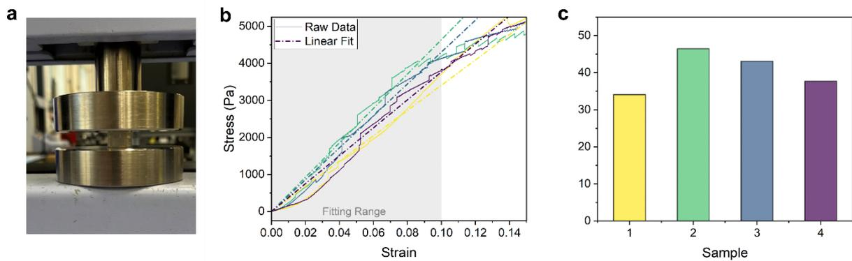
Supplementary Figure 22. Uniaxial compression testing of 2% w/v agarose hydrogels. (a) Experimental setup and sample geometry, (b) linear fits of stress/strain data (to a maximum of 0.1 strain) for four hydrogel samples, and (c) resultant Young's moduli for each sample.
