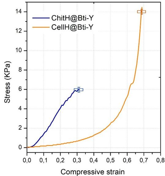
**Figure S2:** Representative stress-strain curve of a CellH and ChitH with active ingredients (Bti and yeasts).
