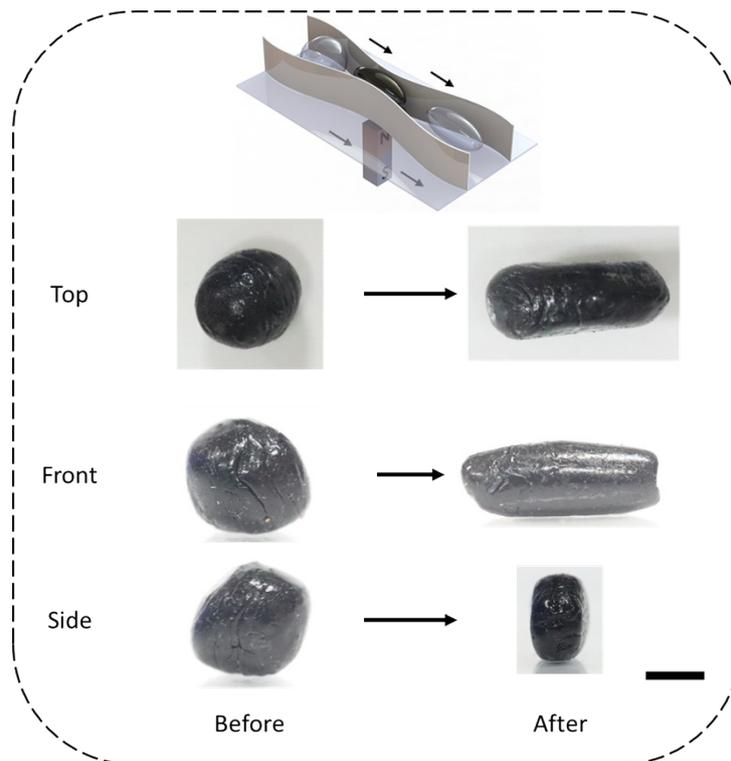
**Figure S4.** Dimensions of a spherical MV before and after passing through a narrow opening. Scale bar, 2 mm.
