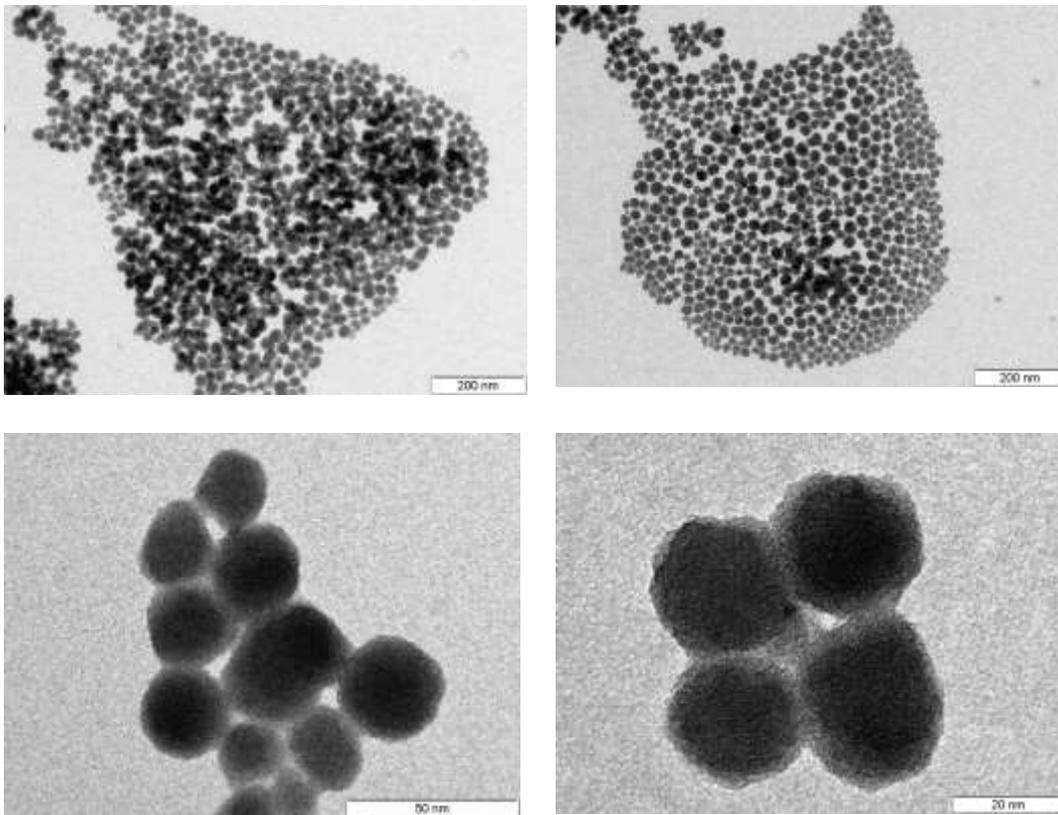
**Figure S4:** TEM images of SiO<sub>2</sub>-APTES sample.
