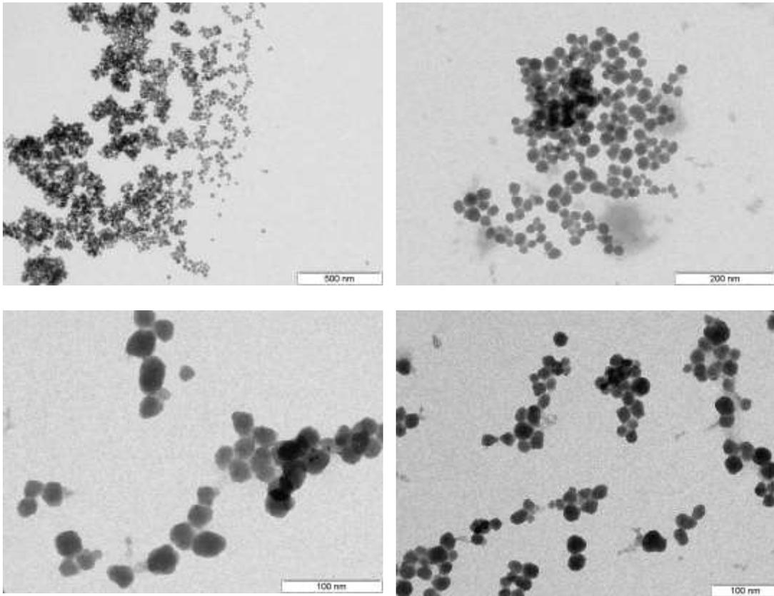
**Figure S6:** TEM images of SiO<sub>2</sub>-HNP\_8 sample.
