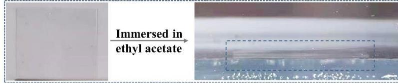
**Fig. S2** The PDMS film made between two PVC boards showed pure swelling without bending in ethyl acetate.
