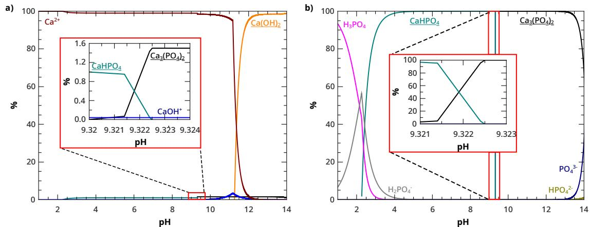
Figure S2. Percentage distribution of (a)  $Ca^{2+}$  and (b)  $PO_4^{3-}$  containing species using  $c_{T,Ca} = 2.0\text{ M}$  and  $c_{T,PO_4} = 26.3\text{ mM}$  concentrations.
