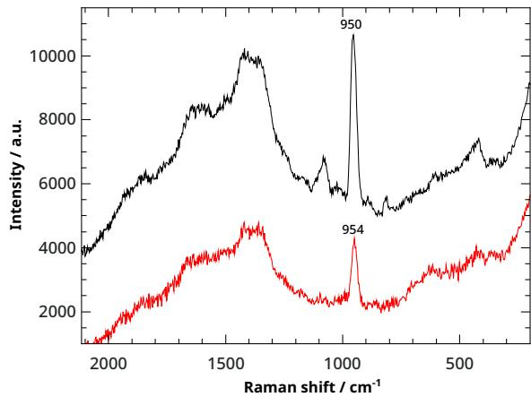
Figure S1. Raman-spectra of dried samples with composition of  $[Na_3PO_4] = 26.3\text{ mM}$  (red) and  $0.263\text{ M}$  (black) in  $0.3\text{ w/V\%}$  alginate. In all cases  $[CaCl_2] = 2.04\text{ M}$ .
