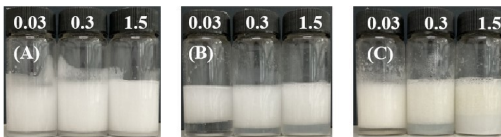
Fig. S4 Digital photographs of Pickering emulsions prepared with (A) n -heptane, (B) ethylacetate and (C) olive oil as oil phase, stabilizing by the 1 wt % TMSNPs in combination with various concentration of CTAB (mmol·L -1 ) as indicated. The photographs were taken 1 h after emulsion preparation.
