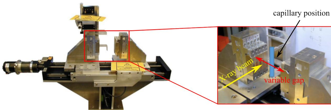
Fig. S1 Permanent magnet setup used for the measurements (left) and the zoom shows the sample position within the Halbach arrangement of magnets (right).
