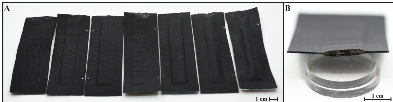
Figure S1: (A) MRJ beams used during experiments. Scaffolding architectures, left to right: none, “blanks” 10 layers, “blanks” 20 layers, “dots” 10 layers, “dots” 20 layers, fibers, and granules. (B) Cross-sectional view of the “dots” 10 layers MRJ beam with MRF seen surrounding and between the layers.
