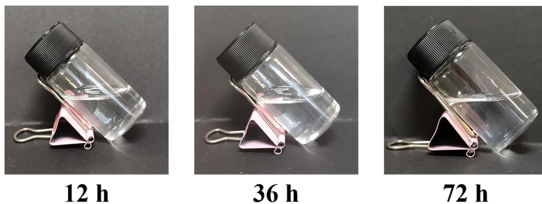
Fig.S1 Digital images of different times after 2 M acetic acid was introduced into PVA aqueous solution.
