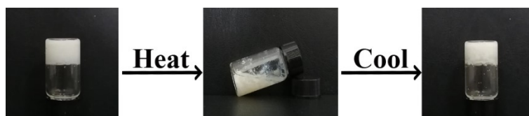
Fig. S8. Illustration for reversible gel-liquid transformation of the L-B-gel triggered by temperature (0.015 g L, 0.1 mol·L -1 B in DMSO, V_{\text{BD}} : V_{\text{D}} : V_{\text{water}} = 1 : 1 : 2 ).
