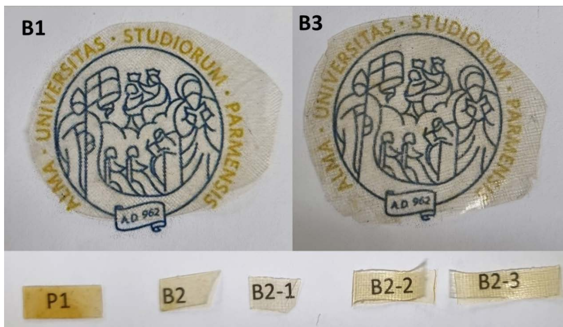
Fig. S4. Images providing the transparency of the films obtained by compression molding.
