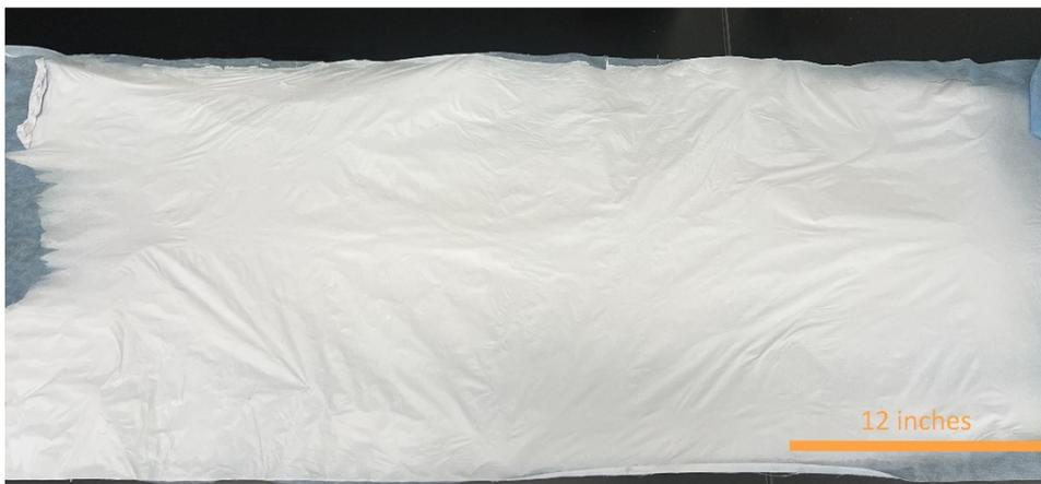
*SI Figure 1. A sample bolt of electrospun, piezoelectric nanofiber material (white) using a production scale Nanospider (needleless) system.*
