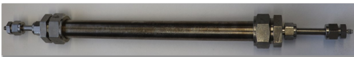
Figure S5: Stainless steel tubular reactor (inner diameter = 21 mm, outer diameter = 25 mm, length = 280 mm).
