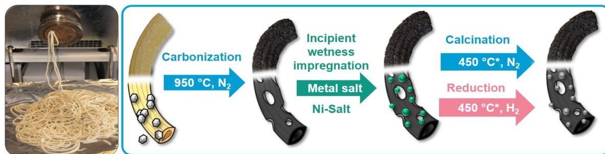
Figure S1 Schematic representation of the catalytic synthesis protocol starting from extrusion (left) followed by carbonization, incipient metal impregnation, calcination and reduction. 2
