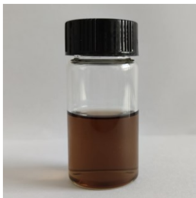
Figure S1. Optical image of the GO dispersion in a mixture of deionized water and ethanol (0.25 mg/ml).
