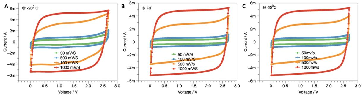
**Figure S2:** The cyclic voltammogram (CV) of on chip supercapacitors at different scan rates and temperatures (a) CV at -20 °C shows device capacitance of 4.8 mF, 4.6 mF, 3 mF and 2.62 mF respectively for 50 mV/S, 100 mV/s, 500 mV/s and 1000 mV/s (b) at room temperature, 8.85 mF, 8.3 mF, 5.75 mF and 4. 75 mF (c) at 60 °C, 10.1 mF, 9.1 mF, 8.1 mF and 5.68 mF respectively.
