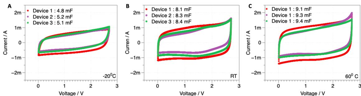
**Figure S3:** Comparison of electrochemical performances of three different on-chip supercapacitors at different temperature ranges (a) CV at  $-20^{\circ}\text{C}$  shows device capacitance of 4.8, 5.2 and 5.3 mF (b) The CV at room temperature with a capacitance of 8.1, 8.3 and 8.4 mF (c) CV at  $60^{\circ}\text{C}$  with a capacitance of 9.1, 9.3 and 9.4 mF. It is worthy to note that for all three devices the capacitance values were around the same at the different temperatures.
